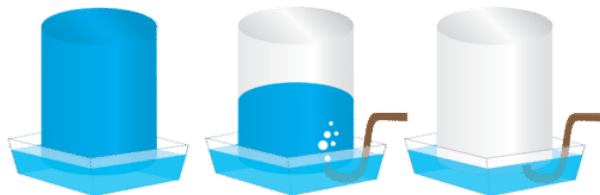
Figure 4.9.2: A gas produced in a chemical reaction can be collected by water displacement.
