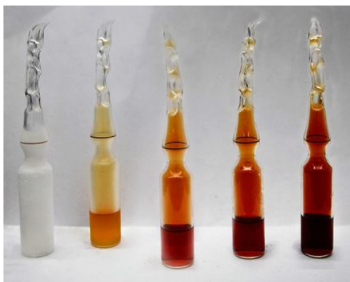
Figure 11.1.1: Dinitrogen tetroxide is a powerful oxidizer that reacts spontaneously upon contact with various forms of hydrazine, which makes the pair a popular propellant combination for rockets. Nitrogen dioxide at -196\text{ }^{\circ}\text{C} , 0\text{ }^{\circ}\text{C} , 23\text{ }^{\circ}\text{C} , 35\text{ }^{\circ}\text{C} , and 50\text{ }^{\circ}\text{C} . ( \text{NO}_2 ) converts to the colorless dinitrogen tetroxide ( \text{N}_2\text{O}_4 ) at low temperatures, and reverts to \text{NO}_2 at higher temperatures. (CC BY-SA 3.0; Eframgoldberg ).
