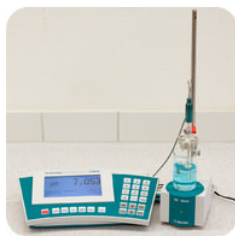
Figure 10.9.1: A pH meter is a laboratory device that provides quick, accurate measurements of the pH of solutions. (CC BY-NC; CK-12)
