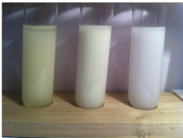
Figure 5.3.1: The three common silver halide precipitates: \text{AgI} , \text{AgBr} and \text{AgCl} (left to right). The silver halides precipitate out of solution, but often form suspensions before settling. (CC BY-SA 3.0; Cychr).
