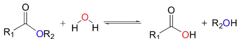
Figure 5.4.1: General reaction scheme of a hydrolysis reaction. FrozenMan, CC BY-SA 4.0, via Wikimedia Commons
