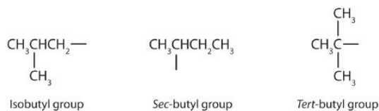
Figure 3.2.6: Common names of butyl substituents.
