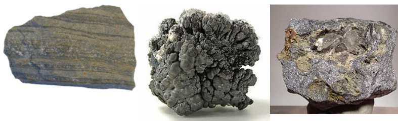
Figure 6.3.1: Three Common Ores. (left) Iron ore, (middle) Manganese ore – psilomelane, and (right) Lead ore – galena and anglesite.
