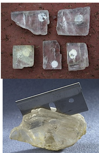
(left) Halite (natural NaCl) crystals easily cleave along planes parallel to the cubic faces. (right) This sample of gypsum ( \text{CaSO}_4 ) is easily cleaved with a razor blade.
