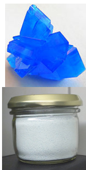
Figure 9.9.1: (left) Crystals of \text{CuSO}_4 \cdot 5\text{H}_2\text{O} . from Stephanb (via Wikipedia). (right) Anhydrous \text{CuSO}_4 after the water was removed.
