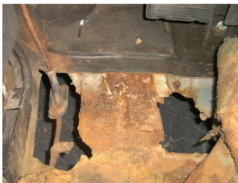
Figure 16.8.4: Rusted out car. Severely rusted floorboards of 1990 Chrysler New Yorker. Car was damaged to the point where it became unsafe to drive. Under the rusting section between the two holes were the two brake lines (Public Domain; Bige1977 via Wikipedia).
