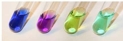
Figure 9.9.4: Color of various Ni(II) complexes in aqueous solution. From left to right, hexaamminenickel(II), tris(ethylenediamine)nickel(II), tetrachloronickelate(II) and hexaaquanickel(II). from LHcheM (via Wikipedia)
