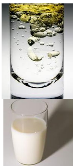
Figure 2.1.1: The phase boundaries in an oil-vinegar salad dressing are easy to see (left), but those in milk are so small that they are only revealed by scattered light (right).
