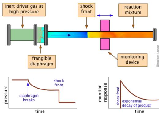
The shock tube itself consists of two sections separated by a breakable diaphragm of metal or plastic. One section is filled with a "driver" gas at a very high pressure, commonly helium, but often mixed with other inert gases to adjust the properties of the shock. The other, longer section of the tube contains the "driven" gas — the reactants — at a low pressure, usually less than 1 atmosphere.
