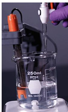
A more modern way of finding an equivalence point is to follow the titration by means of a pH meter. Because it involves measuring the electrical potential difference between two electrodes, this method is known as *potentiometry*. Until around 1980, pH meters were too expensive for regular use in student laboratories, but this has changed; potentiometry is now the standard tool for determining equivalence points.
