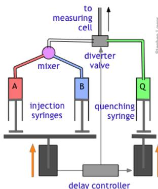
The quenched-flow technique works something like the stopped-flow method described above, with a slightly altered plumbing arrangement. The reactants A and B are mixed and fed directly through the diverter valve to the measuring cell, which is not shown in this diagram. After a set interval that can vary from a few milliseconds to 200 sec or more, the controller activates the quenching syringe and diverter valve, flooding the cell with the quenching solution.
