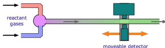
If the distance between the point at which the reaction is initiated and the product detector is known, then the time interval can be found from the flow rate. By varying this distance, the time required to obtain the maximum yield can then be determined.
