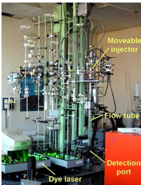
Although this method is very simple in principle, it can be rather complicated in practice, as the illustration shows. Owing to the rather large volumes required, this method is more practical for the study of gas-phase reactions than for solutions, for which the stopped-flow method described below is generally preferred.
