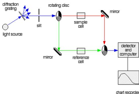
More sophisticated *absorption spectrophotometers* employ two cells (one for the sample and another *reference cell* for the blank). They also allow one to select the particular wavelength range that is most strongly absorbed by the substance under investigation, which can often extend into the near-ultraviolet region.
