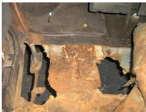
Figure 16.8.4: Rusty out car. Severely rusted floorboards of 1990 Chrysler New Yorker. Car was damaged to the point where it became unsafe to drive. Under the rusting section between the two holes were the two brake lines (Public Domain; Bige1977 via Wikipedia).
