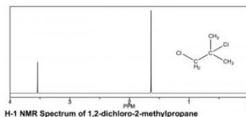
The basic theory of both H-1 and C-13 NMR are the same and, in fact, both spectra can be recorded on the same instrument. The sample is placed in a magnetic field that splits the spin states of the H-1 nuclei; the energy required to flip the nuclei from one spin state to another is detected and is transformed into a spectrum such as the one below.
