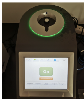
A model of bench top NMR: NMRReady-60
