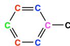
toluene molecule has 5 different sets of carbon atoms (hydrogen atoms are omitted)
