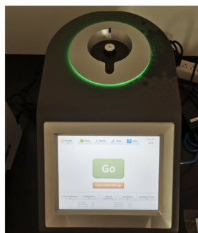
A model of bench top NMR: NMReady-60
