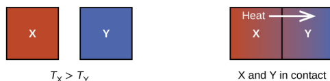
Figure 8.1.4: When two objects at different temperatures come in contact, heat spontaneously flows from the hotter to the colder object. Two separated blocks. One is labeled X and the other labeled Y. The diagram next to it shows the two blocks in contact with one another.
