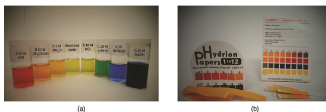
Figure 5.2.3: (a) A universal indicator assumes a different color in solutions of different pH values. Thus, it can be added to a solution to determine the pH of the solution. The eight vials each contain a universal indicator and 0.1-M solutions of progressively weaker acids: HCl (pH = 1), \text{CH}_3\text{CO}_2\text{H} (pH = 3), and \text{NH}_4\text{Cl} (pH = 5), deionized water, a neutral substance (pH = 7); and 0.1-M solutions of the progressively stronger bases: KCl (pH = 7), aniline, \text{C}_6\text{H}_5\text{NH}_2 (pH = 9), \text{NH}_3 (pH = 11), and NaOH (pH = 13). (b) pH paper contains a mixture of indicators that give different colors in solutions of differing pH values. (credit: modification of work by Sahar Atwa)
