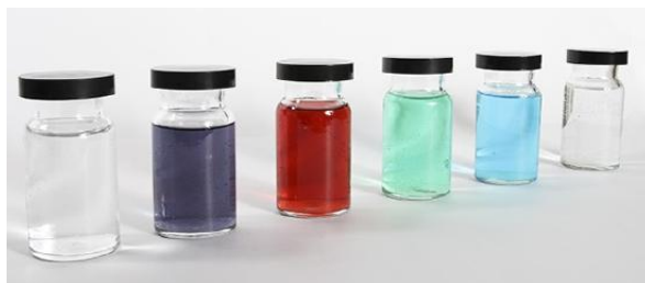
Figure 2.2.1: Metal ions that contain partially filled d subshell usually form colored complex ions; ions with empty d subshell ( d^0 ) or with filled d subshells ( d^{10} ) usually form colorless complexes. This figure shows, from left to right, solutions containing [M(H_2O)_6]^{n+} ions with M = Sc^{3+}(d^0) , Cr^{3+}(d^3) , Co^{2+}(d^7) , Ni^{2+}(d^8) , Cu^{2+}(d^9) , and Zn^{2+}(d^{10}) . (credit: Sahar Atwa)
