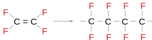
Figure 1.9.2: Polytetrafluoroethylene (also known as Teflon) is formed from the polymerization of tetrafluoroethylene.
