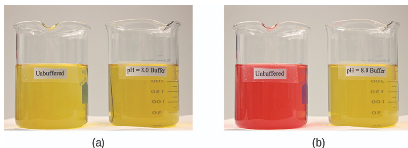
Figure 6.3.1: (a) The unbuffered solution on the left and the buffered solution on the right have the same pH (pH 8); they are basic, showing the yellow color of the indicator methyl orange at this pH. (b) After the addition of 1 mL of a 0.01-M HCl solution, the buffered solution has not detectably changed its pH but the unbuffered solution has become acidic, as indicated by the change in color of the methyl orange, which turns red at a pH of about 4. (credit: modification of work by Mark Ott)
