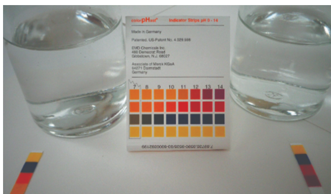
Figure 5.5.1: pH paper indicates that a 0.1-M solution of \text{NH}_3 (left) is weakly basic. The solution has a pOH of 3 ( [\text{OH}^-] = 0.001 M) because the weak base \text{NH}_3 only partially reacts with water. A 0.1-M solution of \text{NaOH} (right) has a pOH of 1 because \text{NaOH} is a strong base (credit: modification of work by Sahar Atwa).
