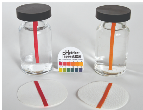
Figure 5.3.1: pH paper indicates that a 0.1-M solution of HCl (beaker on left) has a pH of 1. The acid is fully ionized and [\text{H}_3\text{O}^+] = 0.1 \text{ M} . A 0.1-M solution of \text{CH}_3\text{CO}_2\text{H} (beaker on right) has a pH of 3 ( [\text{H}_3\text{O}^+] = 0.001 \text{ M} ) because the weak acid \text{CH}_3\text{CO}_2\text{H} is only partially ionized. In this solution, [\text{H}_3\text{O}^+] < [\text{CH}_3\text{CO}_2\text{H}] . (credit: modification of work by Sahar Atwa)
