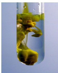
Figure 7.8.2: When a small amount of \text{Na}_2\text{CrO}_4 solution is added to a sample containing \text{Pb}^{2+} ions in water, a bright yellow precipitate of \text{PbCrO}_4 forms. (CC BY-SA 3.0 Unported; PRHaney via Wikipedia).
