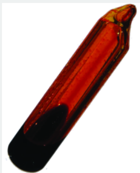
Figure 4.1.4: An equilibrium is pictured between liquid bromine, \text{Br}_2(\text{l}) , the dark liquid, and bromine vapor, \text{Br}_2(\text{g}) , the orange gas. Because the container is sealed, bromine vapor cannot escape and equilibrium is maintained. (credit: http://images-of-elements.com/bromine.php ).
