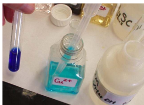
Figure 7.7.1: The Formation of Complex Ions. An aqueous solution of \text{CuSO}_4 consists of hydrated \text{Cu}^{2+} ions in the form of pale blue [\text{Cu}(\text{H}_2\text{O})_6]^{2+} (left). The addition of aqueous ammonia to the solution results in the formation of the intensely blue-violet [\text{Cu}(\text{NH}_3)_4(\text{H}_2\text{O})_2]^{2+} ions, usually written as [\text{Cu}(\text{NH}_3)_4]^{2+} ion (right) because ammonia, a stronger base than \text{H}_2\text{O} , replaces water molecules from the hydrated \text{Cu}^{2+} ion. For a more complete description, see https://www.youtube.com/watch?v=IQNcLH6OZK0 .
