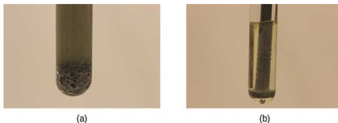
Figure 3.2.1: (a) Iron powder reacts rapidly with dilute hydrochloric acid and produces bubbles of hydrogen gas because the powder has a large total area. (b) An iron nail reacts more slowly.
