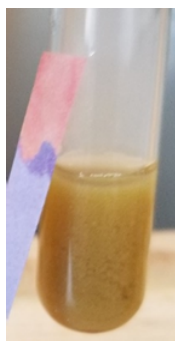
Figure 4.2.2: \text{Sn}^{4+} yellow precipitate confirming the presence of \text{Sn}^{4+} in the test sample.
