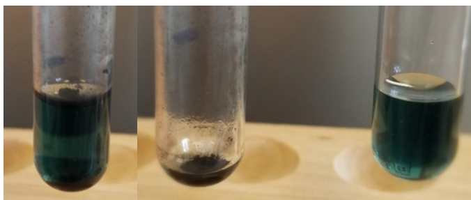
Figure 5.2.1: Group III mixture after heating with HCl solution (right), NiS precipitate (middle), and the supernatant containing \text{Cr}^{3+} and \text{Fe}^{2+} (right) separated by aspiration with the cotton-plug technique after centrifugation.
