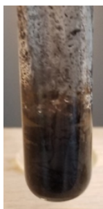
Figure 4.1.1: Mixture of Group II precipitates, i.e., \text{SnS}_2 (yellow), \text{CdS} (yellow-orange), \text{CuS} (Black-brown), and \text{Bi}_2\text{S}_3 (black).
