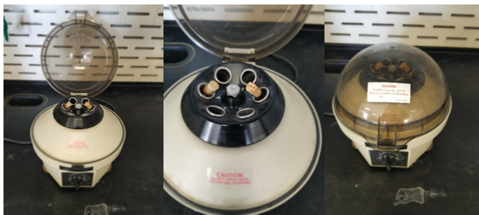
Figure 2.3.2: A laboratory centrifuge machine with the lid open (left), rotor compartment showing test tubes placed across to balance the weight (middle), centrifuge ready to start with a sample loaded, and the lid closed.
