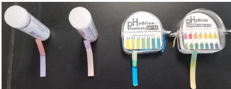
Figure 2.5.1: Illustration of pH measurements, from left to right: i) blue litmus paper turned red at the top end by an alkaline solution, ii) red litmus paper turned blue at the top end by an alkaline solution, iii) short-range pH paper testing a solution of pH \sim 0.5 , and iv) full range pH paper testing a solution at pH \sim 8 .
