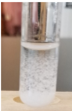
Figure 3.2.2: \text{PbCl}_2 recrystallized upon cooling the hot solution and addition of two drops of 6M HCl.
