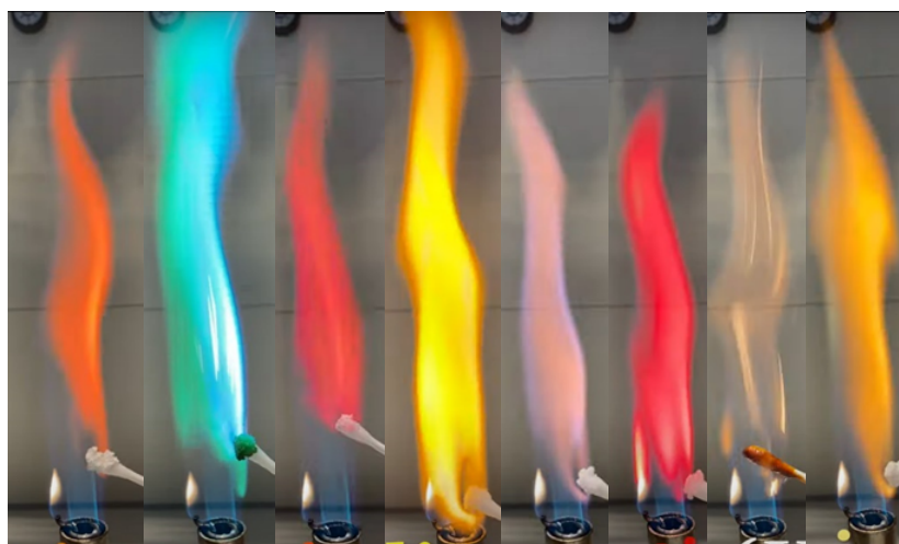
Figure 2.6.3: Flame test colors, from left to right: red \text{CaCl}_2 , blue \text{CuCl}_2 , red \text{LiCl} , yellow \text{NaCl} , purple \text{KCl} , red \text{SrCl}_2 , folder sparkly \text{FeCl}_3 , and yellow-green \text{BaCl}_2 . Source: taken from a YouTube video contributed by Step by Step Science .
