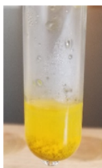
Figure 4.2.4: Yellow precipitate CdS confirming the presence of \text{Cd}^{2+} in the test sample.
