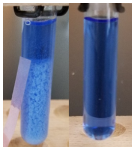
Figure 4.2.7: Confirmation test of copper, i.e., the solution turned dark blue due to [\text{Cu}(\text{NH}_3)_4]^{2+} ions upon turning alkaline with ammonia. The solution is turbid due to \text{Bi}(\text{OH})_3 precipitate (left), and becomes clear after removal of \text{Bi}(\text{OH})_3 by centrifugation (right).
