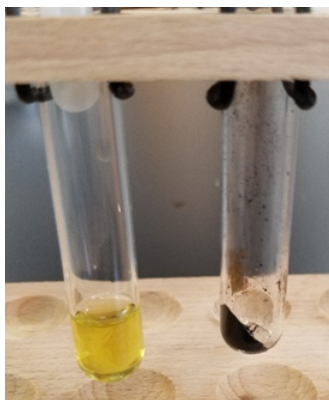
Figure 4.2.1: Supernatant containing [\text{Sn}(\text{OH})_6]^{2-} and [\text{SnS}_3]^{2-} (left test tube) and blackish precipitate (right test tube) containing mixture of CdS (yellow-orange), CuS (Black-brown), and \text{Bi}_2\text{S}_3 (black).
