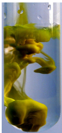
Figure 1.1.1: Precipitation reaction: \text{Pb}(\text{NO}_3)_2(\text{aq}) + 2\text{KI}(\text{aq}) \rightarrow \text{PbI}_2(\text{s})\downarrow + 2\text{KNO}_3(\text{aq}) . source: PRHaney [CC BY-SA ( https://creativecommons.org/licenses/by-sa/4.0/ )].
