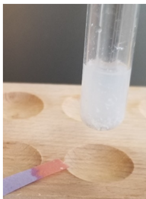
Figure 3.2.4: Confirmation of \text{Ag}^+ : formation of white precipitate upon converting [\text{Ag}(\text{NH}_3)_2(\text{aq})]^+ solution from alkaline to acidic by addition of \text{HNO}_3 .
