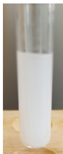
Figure 2.4.3: Precipitate re-suspended in a washing solvent.
