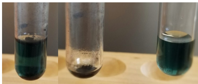
Figure 5.2.1: Group III mixture after heating with HCl solution (right), \text{NiS} precipitate (middle), and the supernatant containing \text{Cr}^{3+} and \text{Fe}^{2+} (left) separated by aspiration with the cotton-plug technique after centrifugation.
