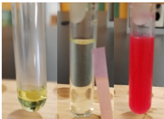
Figure 5.2.3: Clear solution containing [\text{Ni}(\text{NH}_3)_6]^{2+} ions obtained after dissolving NiS in aqua-regia (left), the [\text{NiCl}_4]^{2-} converted to [\text{Ni}(\text{NH}_3)_6]^{2+} by making the solution alkaline by ammonia addition (middle), and red precipitate \text{NiC}_8\text{H}_{14}\text{O}_4 formed by adding dimethylglyoxime to the solution.
