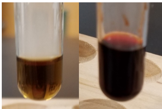
Figure 5.2.6: The \text{Fe}(\text{OH})_3 precipitate dissolved in \text{HCl} (left) and forms deep-red color [\text{FeSCN}]^{2+} by reacting with \text{SCN}^- (right).
