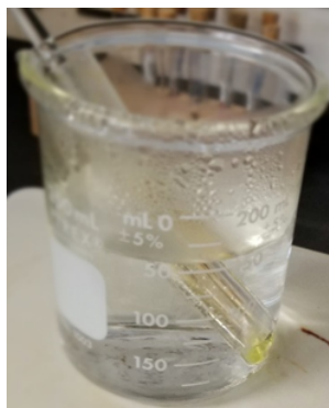
Figure 5.2.2: NiS being dissolved in aqua-regia as [\text{NiCl}_4]^{2-} coordination anion, \text{S}^{2-} oxidized to yellowish S particles, \text{NO}_3^- reduced to NO and then oxidized to brown color gas \text{NO}_2 in the air above the mixture.
