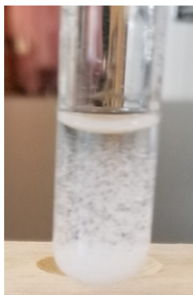
Figure 3.2.2: \text{PbCl}_2 recrystallized upon cooling the hot solution and addition of two drops of 6M HCl.
