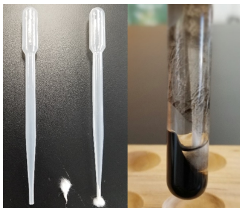
Figure 2.4.2: Cotton plug technique, from left to right: i) a Pasteur pipette, ii) a cotton tuft made pointy at one end, iii) a Pasteur pipette with cotton-plug fitted in the tip, and iv) aspiration from a loosely packed precipitate using cotton plug technique.
