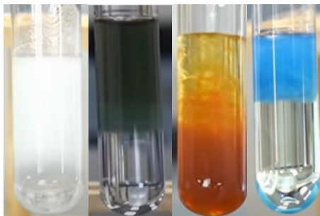
Figure 1.1.3: The precipitates of some insoluble ionic compounds formed by mixing the aqueous solution of appropriate soluble ionic compounds. The precipitates are from left: white Calcium sulfate ( \text{CaSO}_4 ), black Iron(II) hydroxide ( \text{Fe(OH)}_2 ), brown Iron(III) hydroxide ( \text{Fe(OH)}_3 ), and blue Copper(II) hydroxide ( \text{Cu(OH)}_2 ). Note that the precipitate is not yet settled at the bottom of the solution; it is still in suspension form in these examples. Source: https://youtu.be/jltLlzZ6FqU
