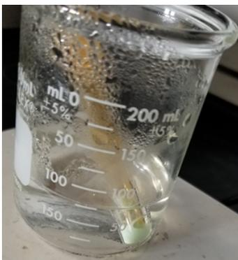
Figure 4.2.5: Yellow sulfur precipitate suspended in the liquid mixture and brown  $\text{NO}_2$  gas above the liquid mixture when  $\text{CuS}$  and  $\text{Bi}_2\text{S}_3$  precipitate is heated with nitric acid.
