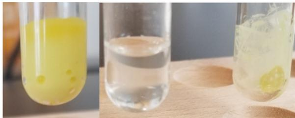
Figure 6.2.2: Selective precipitation of  $\text{BaCrO}_4$  by adding  $\text{CrO}_4^{2-}$  at pH  $\sim 5$  leaving  $\text{Ca}^{2+}$  in the solution(left) and supernatant (middle) separated from precipitate (right) after centrifugation and decantation.
