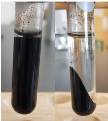
Figure 5.1.2: Group III precipitates, i.e.,  $\text{Cr}(\text{OH})_3(\text{s, gray-green})$ ,  $\text{NiS}(\text{s, black})$ ,  $\text{Fe}_2\text{S}_3(\text{s, yellow-green})$ , and  $\text{FeS}(\text{s, black})$  in the mixture before centrifuge (left) and separated as a pellet at the bottom of the test tube after centrifuge (right).
