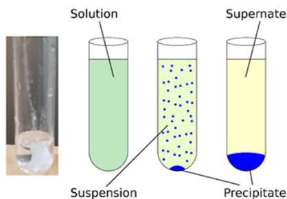
Figure 2.1.2: Formation of a milky-white  $\text{AgCl}$  precipitate upon addition of  $\text{HCl}$  to  $\text{AgNO}_3$  solution and illustration of a solution, suspension, and precipitation. (Attributes for the illustration: [ZabMilenko](#): [original](#)[ZooFari](#): [vectorMrmw](#): [optimized](#), [multilang](#), [CC0](#), via [Wikimedia Commons](#))
