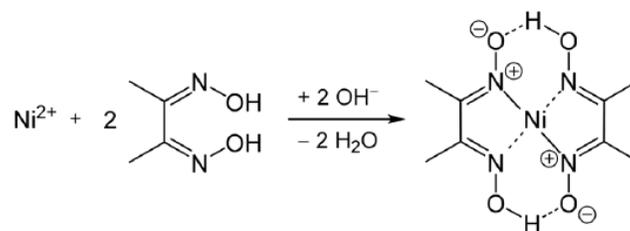
Figure 5.2.4: Reaction of  $\text{Ni}^{2+}$  with dimethyl glyoxime forming a red color coordination compound in confirmation test of nickel ion. Four coordinate covalent bonds formed in the complex between nickel and nitrogen atoms by the donation of lone pair of electrons on nitrogen are shown in the product.
