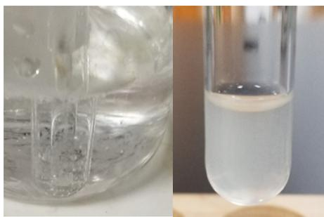
Figure 5.2.7: After oxidizing  $\text{CrO}_4^{2-}$  to  $\text{Cr}^{3+}$ , hydrogen peroxide is destroyed by heating which can be observed as oxygen gas bubbles leaving the mixture (left), and  $\text{Cr}^{3+}$  is confirmed by forming gray-green  $\text{Cr}(\text{OH})_3$  precipitate (right). Note:  $\text{Cr}(\text{OH})_3$  is usually formed in a very small amount at this stage making it difficult to detect.
