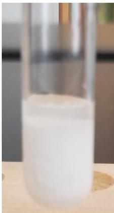
Figure 6.1.1: Group IV precipitates,  $\text{CaCO}_3$  and  $\text{BaCO}_3$ .
