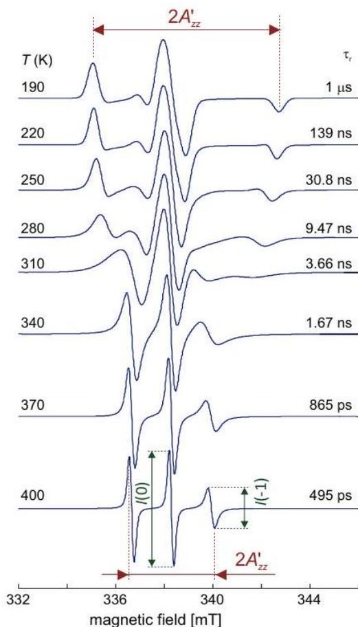
Figure 10.4: Simulation of X-band CW EPR spectra of an isotropically tumbling nitroxide radical for different rotational correlation times. A rotational correlation time of  $\tau_r$  at and an activated process with activation energy of  $E_a$  were assumed, close to parameters observed for TEMPO in a synthetic polymer.
