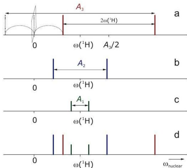
Figure 4.6: Schematic ENDOR (nuclear frequency) spectrum of the phenyl radical at an X-band frequency where . (a) Subspectrum of the two equivalent ortho protons. The strong-coupling case applies. (b) Subspectrum of the two equivalent meta protons. The weak-coupling case applies. (c) Subspectrum of the para proton. The weak-coupling case applies. (d) Complete spectrum.
