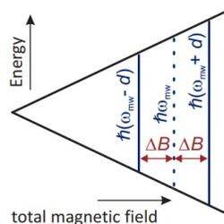
Figure 9.1: Resonance frequency shift of an observer spin (blue transitions) by the change  $\pm\Delta B$  in local magnetic field that arises upon a flip of a second spin that is dipole-dipole coupled to the observer spin. Compare Fig. 5.3 for the local field picture.
