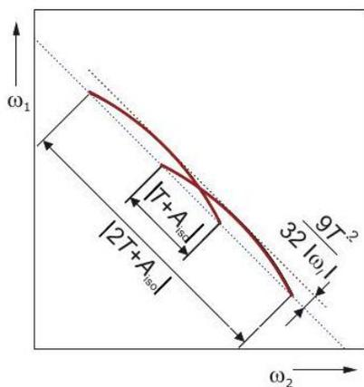
Figure 8.6: Schematic HSCORE spectrum for a proton with an axial hyperfine tensor with anisotropy  $T$  and isotropic component  $A$ . The correlation peaks from different orientations form curved ridges (red). Curvature is the stronger the larger the anisotropy is and the ratio of squared anisotropy to the nuclear Zeeman frequency determines the maximum shift with respect to the anti-diagonal.
