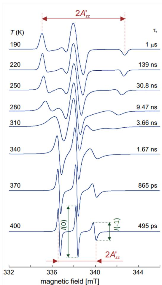
Figure 10.4: Simulation of X-band CW EPR spectra of an isotropically tumbling nitroxide radical for different rotational correlation times  $\tau_r$ . A rotational correlation time of  $1\mu\text{ s}$  at 190 K and an activated process with activation energy of  $22.9\text{ kJ mol}^{-1}$  were assumed, close to parameters observed for TEMPO in a synthetic polymer.
