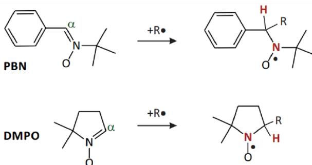
Figure 10.8: Reaction of the commonly used spin traps phenylbutylnitron (PBN) and 5,5-dimethyl-1-pyrroline N-oxide (DMPO) with unstable radicals  $\text{R}\bullet$ . Hyperfine couplings of the  $^{14}\text{N}$  and  $\text{H}^\alpha$  atom of the formed nitroxide (red) as well as the  $g$  value of the nitroxide provide fingerprint information on the type of radical  $\text{R}\bullet$ .
