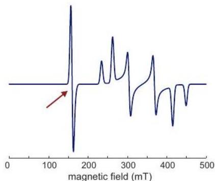
Figure 5.7: CW EPR spectrum of the excited naphthalene triplet at thermal equilibrium (simulation at an  $\nu$ -band frequency of ). The red arrow marks the half-field signal, which corresponds to the formally forbidden double-quantum transition .
