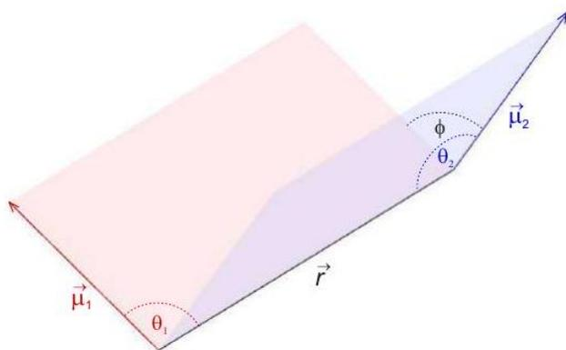
Figure 5.2: Geometry of two magnetic point dipoles in general orientation. Angles  $\theta_1$  and  $\theta_2$  are included between the respective magnetic moment vectors or  $\mu_1$  and  $\mu_2$  and the distance vector between the point dipoles. Angle  $\phi$  is the dihedral angle.
