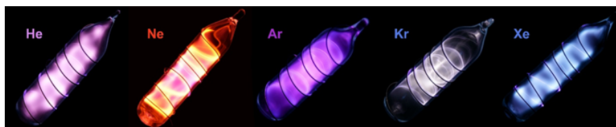
Figure 2.4.6: Glowing noble gases in glass vials with low pressure inside. Power supply: 5 kV, 20 mA, 25 kHz. Source: New work Alchemist-hp (talk) www.pse-mendejew.de); original single images: Jurii, http://images-of-elements.com . / CC BY ( https://creativecommons.org/licenses/by/3.0 )
