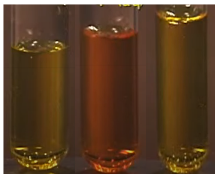
Figure 6.4.4: Demonstration of effect of concentration change on chemical equilibrium: \text{Cr}_2\text{O}_7^{2-}(\text{aq, brown}) + \text{H}_2\text{O}(\text{l}) \rightleftharpoons 2\text{CrO}_4^{2-}(\text{aq, yellow}) + 2\text{H}^+(\text{aq}) . Addition of \text{H}^+ to the tube on left by adding \text{HNO}_3 shifts the equilibrium to left making more of brown \text{Cr}_2\text{O}_7^{2-} shown in the middle tube. Removal of \text{H}^+ by adding a base \text{NaOH} shift the reaction to the right making more of yellow \text{CrO}_4^{2-} shown in right most tube. Source: NCSSMDistanceEd / CC BY ( https://creativecommons.org/licenses/by/3.0 )
