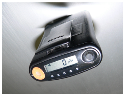
Figure 8.4.6: View of readout on an electronic personal dosimeter. The clip is used to attach it to the wearer's clothing. Source: Rama / CC BY-SA 2.0 FR ( https://creativecommons.org/licenses...2.0/fr/deed.en )
