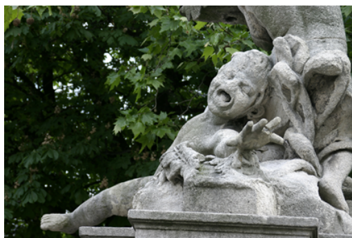
Figure 6.6.7: PEfect of acid rain on monuments. Source: Nino Barbieri / CC BY-SA ( http://creativecommons.org/licenses/by-sa/3.0/ )
