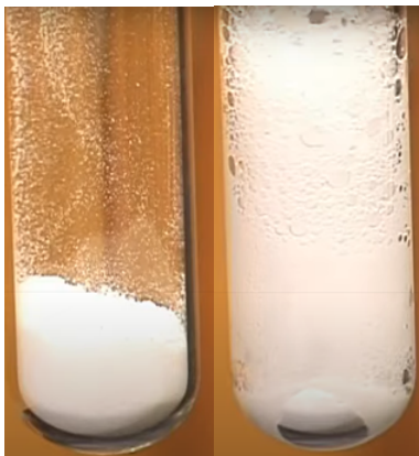
Figure 6.7.2: The reaction of sodium carbonate with HCl. Before and after HCl addition. Carbon dioxide bubbles out after HCl addition. Source: NCSSM, 05/18/20, https://youtu.be/TJYOxGHNTzg , CC BY 3.0
