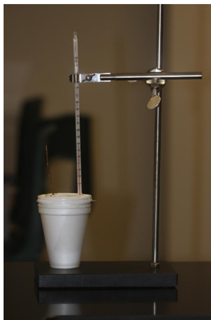
Figure 1.8.4: Photo of coffee cup calorimeter set. Source: Community College Consortium for Bioscience Credentials / CC BY ( https://creativecommons.org/licenses/by/3.0 )
