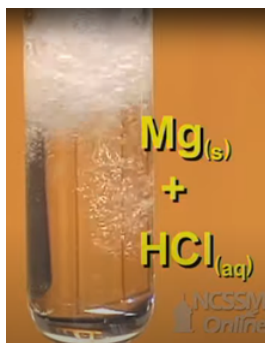
Figure 4.4.4: Single replacement reaction of magnesium with hydrochloric acid producing hydrogen gas: \text{Mg(s)} + 2\text{HCl(aq)} \rightarrow \text{MgCl(aq)} + \text{H}_2(\text{g})\uparrow Source: taken from NCSSM online youtube video, 05/18/20, https://www.youtube.com/watch?v=OBdgeJFzSec
