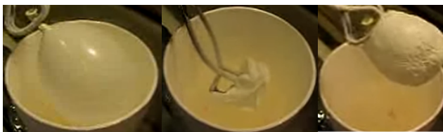
Figure 7.3.1: Air balloon (left) shrinks when its temperature is decreased by submerging in liquid nitrogen (middle) and re-expands when returned to room temperature condition (right). Source: Ryan Poling aka expictura on Flickr. https://en.Wikipedia.org/wiki/File:Nitrogen.ogv#file , CC BY 2.0
