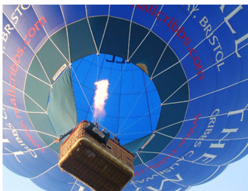
Figure 7.3.3: A hot air balloon seen from a view directly below. The burner, or flame, is firing into the envelope above. The warm air is less dense than the atmospheric air which makes the balloon rise in the air. Source: Arpingstone at English Wikipedia / Public domain.
