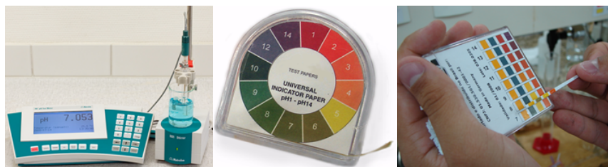
Figure 6.6.1: pH/Ion Meter (left) and universal pH indicator papers (middle and right). Source: Datamax / Public domain; Bordercolleiez / CC0; Fredquintao~commonswiki, CC-BY-SA-2.5.
