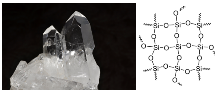
Figure 3.1.3: Quartz crystal composed of SiO 2 , and an illustration of covalent bonds in a giant molecule of SiO 2 . Source: Parent Géry, Public domain, via Wikimedia Commons, and Roland Mattern / Public domain
