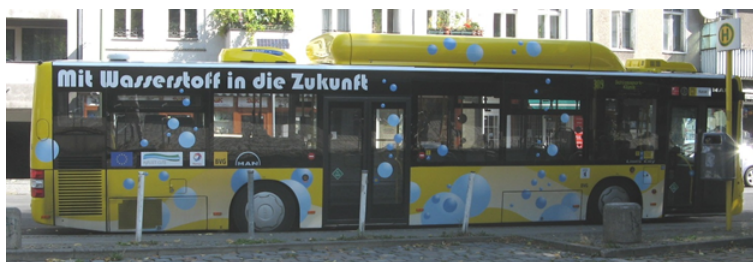
Figure 4.4.2: Berlin public bus using hydrogen as a fuel in an internal combustion engine (ICE). Hydrogen is stored in ten pressure cylinders of 50 kg of hydrogen at 350 bar. Reaction: \text{2H}_2 + \text{O}_2 \rightarrow 2\text{H}_2\text{O} + heat. Source: StralsundByzantion / CC BY-SA ( https://creativecommons.org/licenses/by-sa/3.0 )
