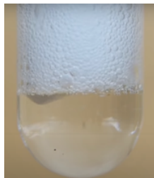
Figure 6.7.1: Mg reacting with HCl and \text{H}_2 gas bubbling out. Source: https://youtu.be/cpy_Zh-8sKA , CC BY
