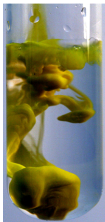
Figure 5.2.7: Precipitation reaction: \text{Pb}(\text{NO}_3)_2(\text{aq}) + 2\text{KI}(\text{aq}) \rightarrow \text{PbI}_2(\text{s})\downarrow + 2\text{KNO}_3(\text{aq}) . source: PRHaney [CC BY-SA ( https://creativecommons.org/licenses/by-sa/3.0 )]
