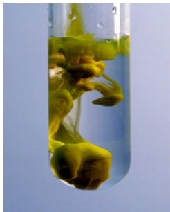
Figure 4.4.8: Lead (II) iodide precipitates when potassium iodide is mixed with lead (II) nitrate: \text{Pb}(\text{NO}_3)_2(\text{aq}) + 2\text{NaI}(\text{aq}) \longrightarrow 2\text{NaNO}_3(\text{aq}) + \text{PbI}_2(\text{s})\downarrow Source: PRHaney / CC BY-SA ( https://creativecommons.org/licenses/by-sa/3.0 )
