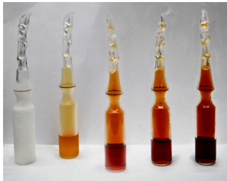
Figure 6.4.7: Increase in temperature shifts the equilibrium in the endothermic direction producing more of the colored \text{NO}_2 in the following equilibrium: \text{N}_2\text{O}_4(g, \text{colorless}) + \text{Heat} \rightleftharpoons 2\text{NO}_2(g, \text{brown}) . An overlay of the same 99.9% pure \text{NO}_2/\text{N}_2\text{O}_4 sealed in an ampoule. From left to right -196\text{ }^\circ\text{C} , 0\text{ }^\circ\text{C} , 23\text{ }^\circ\text{C} , 35\text{ }^\circ\text{C} , 50\text{ }^\circ\text{C} . Source: Eframgoldberg / CC BY-SA ( https://creativecommons.org/licenses/by-sa/3.0 )
