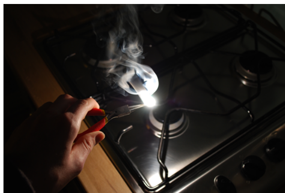
Figure 4.4.5: An image of Ignited Magnesium burning in the air in normal conditions. Yannickcosta1, CC BY SA3, https://commons.wikimedia.org/wiki/File:Magburn1.jpg
