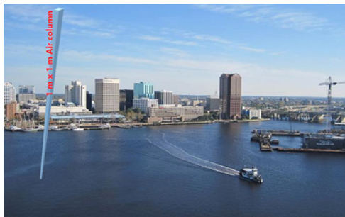
Figure 7.1.2: Illustration of an air column of 1m x 1m base and height covering the entire atmosphere of the earth. Modified from: http://wikimapia.org/8706099/Norfolk.../photo/1606686
