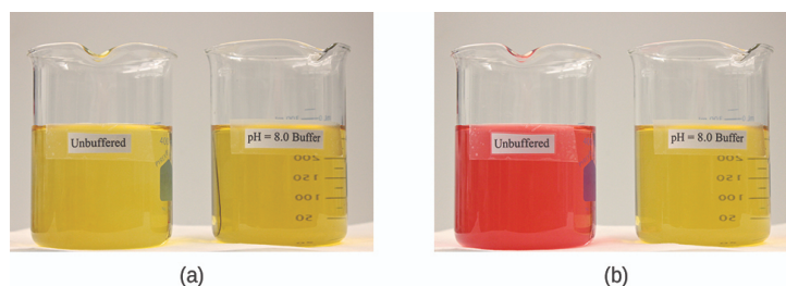
Figure 1. (a) The unbuffered solution on the left and the buffered solution on the right have the same pH (pH 8), showing the yellow color of the indicator methyl orange. (b) After the addition of 1 mL of a 0.01-M HCl solution, the buffered solution pH has not changed detectably. The unbuffered solution has become acidic, as indicated by the red color of the methyl orange, which turns red at a pH of about 4. (credit: modification of work by Mark Ott)
