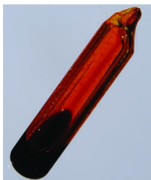
Figure 4. Sample of bromine in a sealed glass tube. Liquid bromine is in the bottom of the tube with gaseous bromine above it.
