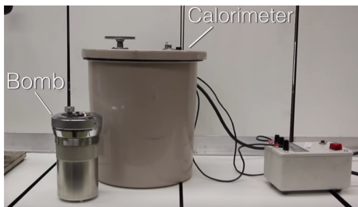
Figure 3. Reactants are added to the stainless steel “bomb”, which is then placed into a water bath inside the calorimeter. Reaction is initiated by brief electric heating and both the bomb and the surrounding water exchange energy with the reaction system. The calorimeter is well insulated so the only energy transfers are between the reaction, the bomb, and the water. The heat transfer of energy can be calculated from the temperature change of bomb and water.
