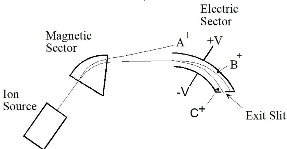
Figure 4.3.1: Reverse Geometry Double Focusing Mass Spectrometer.  $A^+$  is a  $100.00\ m/z$  ion,  $B^+$  is a  $50.00\ m/z$  ion and  $C^+$  is a  $50.01\ m/z$  ion.  $A^+$  is rejected by the magnetic sector because of its greater momentum.  $B^+$  and  $C^+$  are not resolved by the magnetic sector because they have the same momentum. To have the same momentum, however,  $B^+$  must have a more kinetic energy than  $C^+$ . As a result the electric sector separates these two ions.
