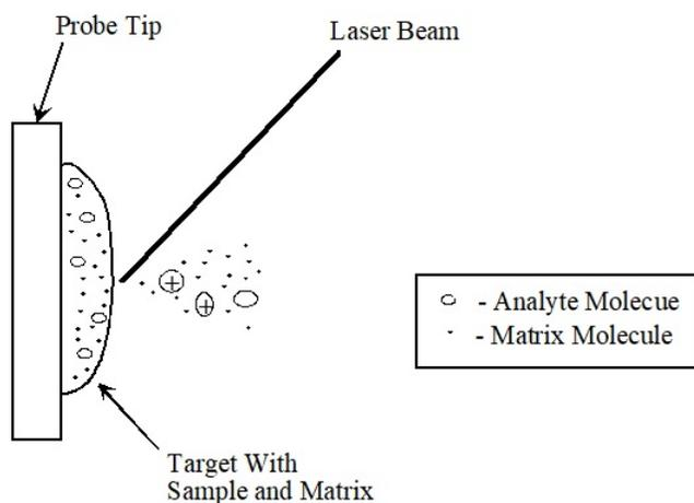
Figure 3.4.1 : MALDI Ionization Target with Sample and Matrix
