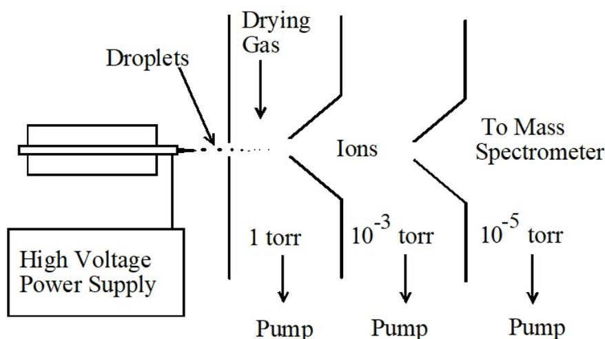
Figure 3.3.1: Electrospray Ionization Source
