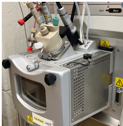
Figure 5.2.1: Electrospray Source
