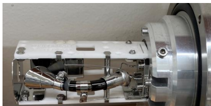
Figure 5.4.1: Electron Multiplier.
