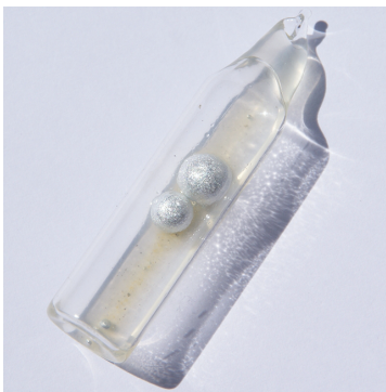
Figure 18.1.3: To prevent contact with air and water, potassium for laboratory use comes as sticks or beads stored under kerosene or mineral oil, or in sealed containers. (credit: Potassium [images-of-elements.com])
