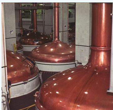
Figure 3.2.3: An oxide of carbon is removed from these fermentation tanks through the large copper pipes at the top. (credit: "Dual Freq"/Wikimedia Commons)
