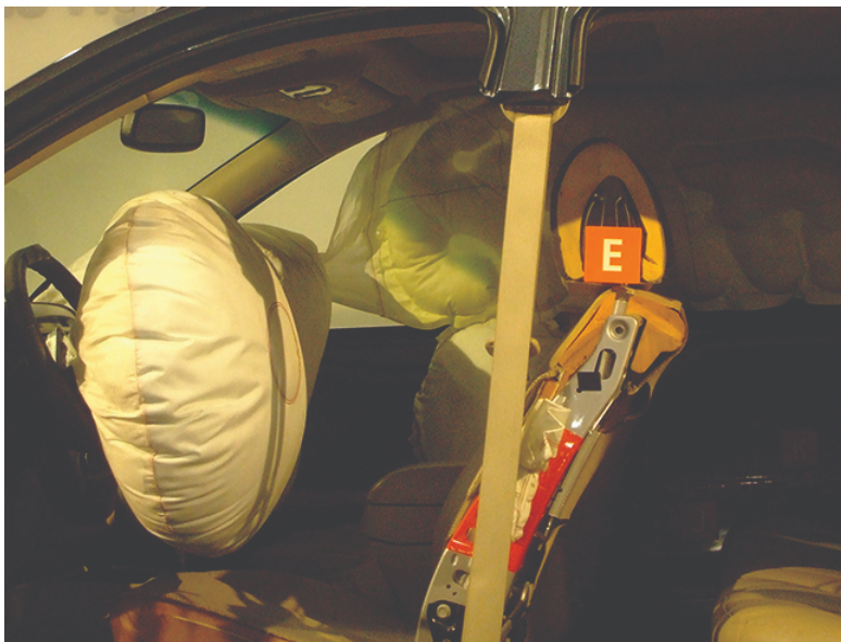
Figure 4.4.3: Airbags deploy upon impact to minimize serious injuries to passengers. (credit: Jon Seidman)
