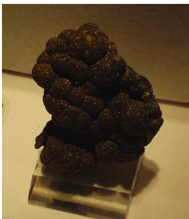
Figure 19.1.8: Blister copper is obtained during the conversion of copper-containing ore into pure copper. (credit: "Tortie tude"/Wikimedia Commons)
