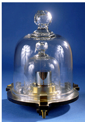
Figure 1.4.2: This replica prototype kilogram is housed at the National Institute of Standards and Technology (NIST) in Maryland. (credit: National Institutes of Standards and Technology).
