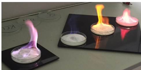
Figure 18.1.4: Colored flames from strontium, cesium, sodium and lithium (from left to right). Picture courtesy of the Claire Murray and Annabelle Baker from the Diamond Light Source.
