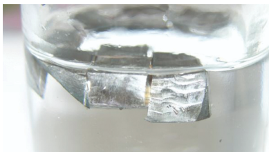
Figure 18.1.2: Lithium floats in paraffin oil because its density is less than the density of paraffin oil.
