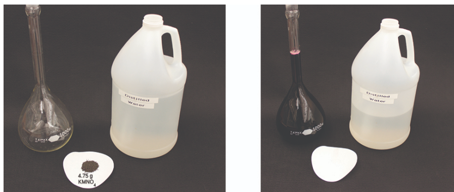
Figure 3.3.3: A solution of KMnO_4 is prepared by mixing water with 4.74 g of KMnO_4 in a flask. (credit: modification of work by Mark Ott)
