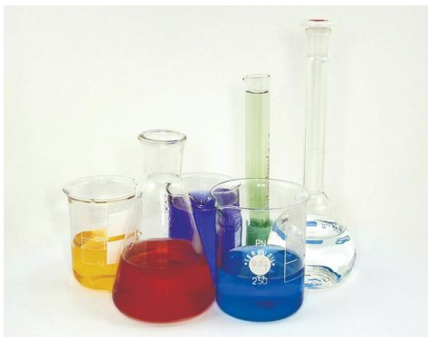
Figure 18.3.4: Laboratory glassware, such as Pyrex and Kimax, is made of borosilicate glass because it does not break when heated. The inclusion of borates in the glass helps to mediate the effects of thermal expansion and contraction. This reduces the likelihood of thermal shock, which causes silicate glass to crack upon rapid heating or cooling. (credit: "Tweenk"/Wikimedia Commons)
