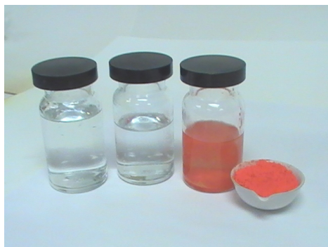
Figure 18.11.2: Solid \text{HgI}_2 forms when solutions of \text{KI} and \text{Hg}(\text{NO}_3)_2 are mixed. (credit: Sahar Atwa).
