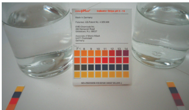
Figure 14.3.5: pH paper indicates that a 0.1-M solution of \text{NH}_3 (left) is weakly basic. The solution has a pOH of 3 ( [\text{OH}^-] = 0.001 \text{ M} ) because the weak base \text{NH}_3 only partially reacts with water. A 0.1-M solution of \text{NaOH} (right) has a pOH of 1 because \text{NaOH} is a strong base (credit: modification of work by Sahar Atwa).
