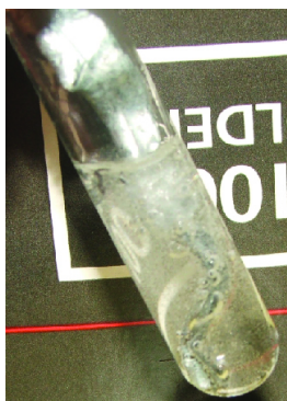
Figure 18.1.6: Zinc is an active metal. It dissolves in hydrochloric acid, forming a solution of colorless Zn 2+ ions, Cl - ions, and hydrogen gas.
