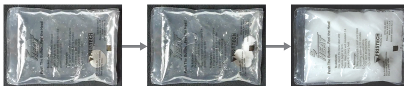
Figure 11.4.10: This hand warmer produces heat when the sodium acetate in a supersaturated solution precipitates. Precipitation of the solute is initiated by a mechanical shockwave generated when the flexible metal disk within the solution is “clicked.” (credit: modification of work by “Veleta”/Wikimedia Commons)
