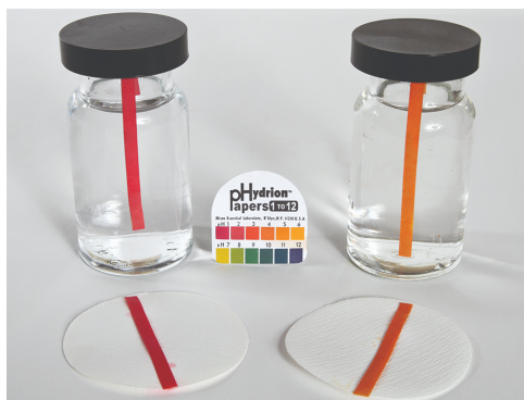
Figure 14.3.4: pH paper indicates that a 0.1-M solution of HCl (beaker on left) has a pH of 1. The acid is fully ionized and [\text{H}_3\text{O}^+] = 0.1 \text{ M} . A 0.1-M solution of \text{CH}_3\text{CO}_2\text{H} (beaker on right) has a pH of 3 ( [\text{H}_3\text{O}^+] = 0.001 \text{ M} ) because the weak acid \text{CH}_3\text{CO}_2\text{H} is only partially ionized. In this solution, [\text{H}_3\text{O}^+] < [\text{CH}_3\text{CO}_2\text{H}] . (credit: modification of work by Sahar Atwa)
