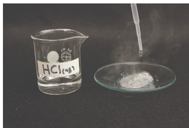
Figure 18.5.2: The reaction of iron with an acid produces hydrogen. Here, iron reacts with hydrochloric acid. (credit: Mark Ott)
