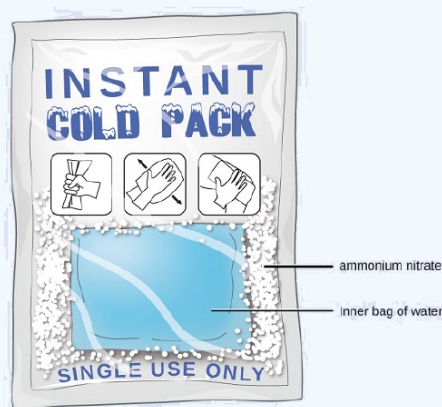
Figure 2.8.5: An instant cold pack consists of a bag containing solid ammonium nitrate and a second bag of water. When the bag of water is broken, the pack becomes cold because the dissolution of ammonium nitrate is an endothermic process that removes thermal energy from the water. The cold pack then removes thermal energy from your body.
