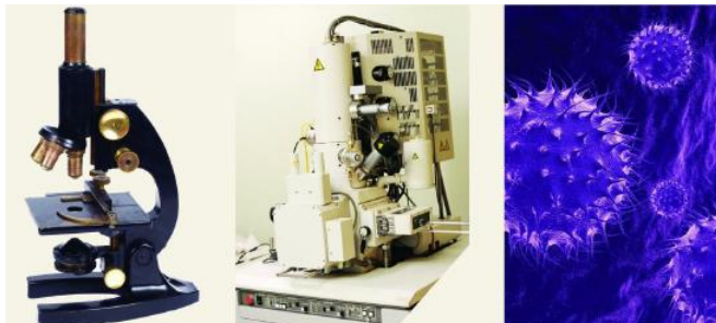
Figure 4.1.1 Microscopes © Thinkstock (a) A simple light microscope can magnify up to 1,500 times. (b) An electron microscope can magnify up to 1,000,000 times. (c) Flu viruses imaged by an electron microscope. The virus is about 100 nm in diameter.
