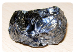
Figure 3.7.3: Silicon. (Credit: User:Enricoros/Wikipedia; Source: http://commons.wikimedia.org/wiki/File:SiliconCroda.jpg (opens in new window); License: Public Domain)
