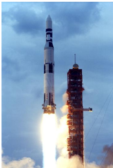
Figure 9.1.1: Saturn V SA-513 lifts off to boost the Skylab Orbital Workshop into Earth orbit. It takes a lot of energy to launch a rocket into space. The Saturn V rocket used five of the most powerful engines ever built to take its initial step into orbit. (Public Domain; NASA)
