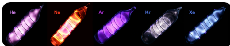
Figure 4.3.2: Gas discharge tubes are enclosed glass tubes filled with a gas at low pressure, through which an electric current is passed. Electrons in the gaseous atoms first become excited, and then fall back to lower energy levels, emitting light of a distinctive color in the process. Shown are gas discharge tubes of helium, neon, argon, krypton, and xenon. (Credit: User:Jurii/Wikimedia Commons, Heinrich Pniok (Wikimedia: Alchemist-hp); Source: Commons Wikimedia, Glowing noble gases (opens in new window) [commons.wikimedia.org]; License: CC by 3.0 (opens in new window))
