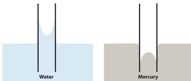
Figure [Math Processing Error]: Capillary Action. (a) Capillary rise is seen when adhesion is strong, such as with water in a thin glass tube. (b) Capillary depression is seen when cohesive forces are stronger than adhesive forces, such as with mercury and thin glass tubes.
