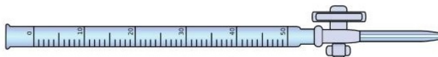
Figure 14.5.1 Equipment for Titrations. A burette is a type of liquid dispensing system that can accurately indicate the volume of liquid dispensed.
