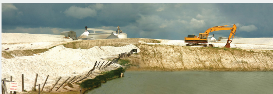
Figure [Math Processing Error]: Salt Mining © Thinkstock. Salt mining can be at the surface or below ground. Here salt is mined from surface deposits. Part of the processing facility can be seen in the background.
