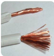
Figure 3.5.4: Copper wire exposed. (Credit: Scott Ehardt; Source: http://commons.wikimedia.org/wiki/File:Stranded_lamp_wire.jpg (opens in new window); License: Public Domain)
