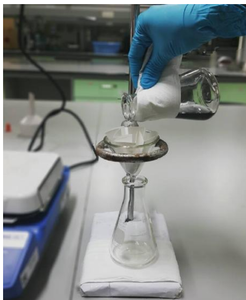
Figure 1.2.4.4: Filtration for the separation of solids from a hot solution. (CC BY-SA 4.0; Suman6395).
