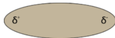
Figure 4.8.6: A dipole is any molecule with a positive end and a negative end, resulting from unequal distribution of electron density throughout the molecule.
