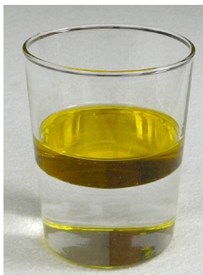
Figure 9.2.2: Water (clear liquid) and oil (yellow) do not form liquid solutions. (CC BY-SA 1.0 Generic; Victor Blacus)
