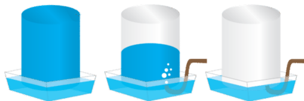
Figure 7.8.2: A gas produced in a chemical reaction can be collected by water displacement.
