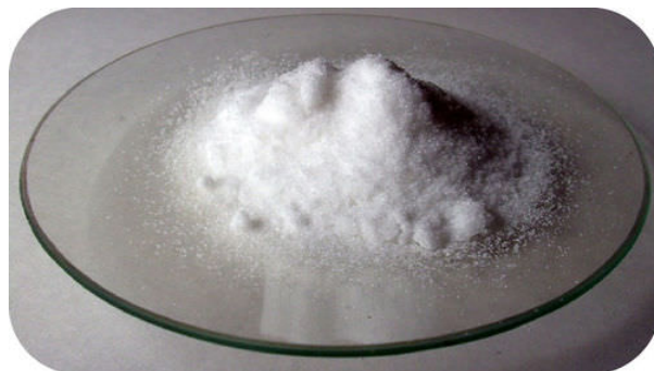
Figure 9.4.5: Calcium nitrate is a typical ionic compound. In an aqueous solution, it dissociates into calcium ions and nitrate ions.
