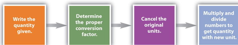
Figure 5.3.1.2 A Flowchart Illustrating the Steps in Performing a Unit Conversion. When performing many unit conversions, the same logical steps can be taken.
