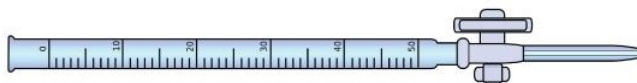
Figure 11.9.1: Equipment for Titrations. A burette is a type of liquid dispensing system that can accurately indicate the volume of liquid dispensed.
