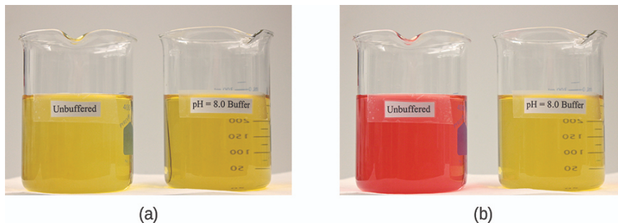
Figure 11.8.1: (a) The unbuffered solution on the left and the buffered solution on the right have the same pH (pH 8); they are basic, showing the yellow color of the indicator methyl orange at this pH. (b) After the addition of 1 mL of a 0.01-M HCl solution, the buffered solution has not detectably changed its pH but the unbuffered solution has become acidic, as indicated by the change in color of the methyl orange, which turns red at a pH of about 4. (credit: modification of work by Mark Ott)
