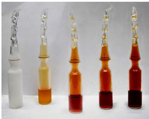
Figure 10.4.1: Dinitrogen tetroxide is a powerful oxidizer that reacts spontaneously upon contact with various forms of hydrazine, which makes the pair a popular propellant combination for rockets. Nitrogen dioxide at -196\text{ }^\circ\text{C} , 0\text{ }^\circ\text{C} , 23\text{ }^\circ\text{C} , 35\text{ }^\circ\text{C} , and 50\text{ }^\circ\text{C} . ( \text{NO}_2 ) converts to the colorless dinitrogen tetroxide ( \text{N}_2\text{O}_4 ) at low temperatures, and reverts to \text{NO}_2 at higher temperatures. (CC BY-SA 3.0; Eframgoldberg ).
