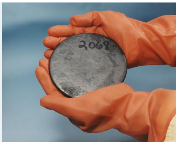
Figure 2.5.3: A billet of highly enriched uranium that was recovered from scrap processed at the Y-12 National Security Complex Plant. Original and unrotated.
