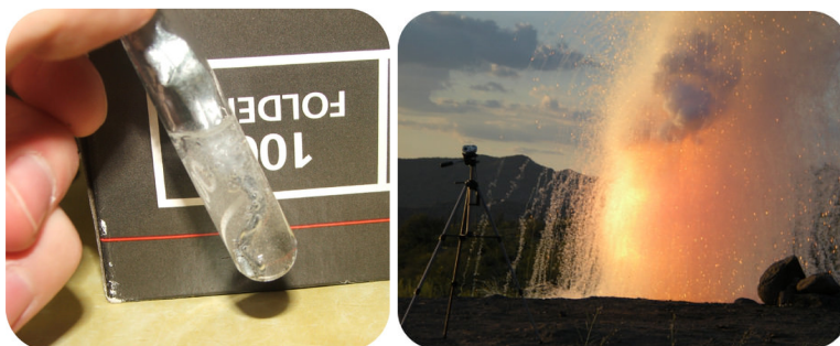
Figure 6.1.2: (First image) Zinc metal reacts with hydrochloric acid to give off hydrogen gas in a single-displacement reaction. (Second image) Sodium metal reacts vigorously with water, giving off hydrogen gas. A large piece of sodium will often generate so much heat that the hydrogen will ignite.
