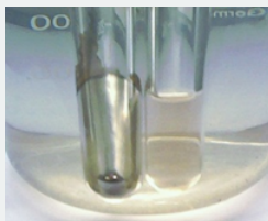
Figure 4.9.3: Tollens' test for aldehydes: left side positive (silver mirror formed) and right side negative. (Copyright; FK1954, Public domain, via Wikimedia Commons)
