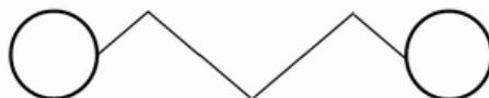
Figure IV.2.B. Two masses connected by a compressible spring can undergo harmonic/oscillatory back-and-forth motions. Click on the image to see the action.
