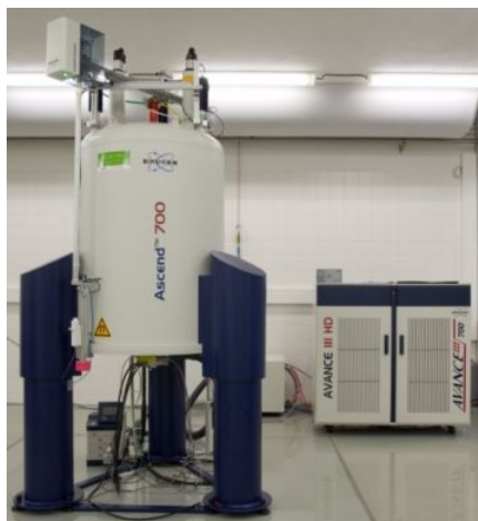
Figure V.I.B A modern NMR spectrometer: Bruker Avance III HD (a cabinet on the background) equipped with a 16.4 Tesla (700 MHz, ^1\text{H} frequency) superconducting magnet (a large cylinder on three vibration-canceling suspension legs).
