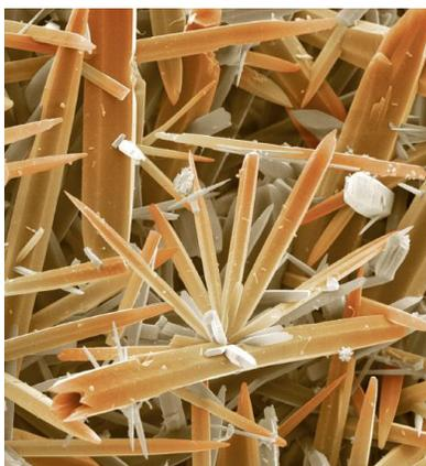
**Scanning electron micrograph of kettle scale.** Hard water is a solution that consists largely of calcium and magnesium carbonate in  $\text{CO}_2$ -rich water. When the water is heated,  $\text{CO}_2$  gas is released, and the carbonate salts precipitate from solution and produce a solid called *scale*.
