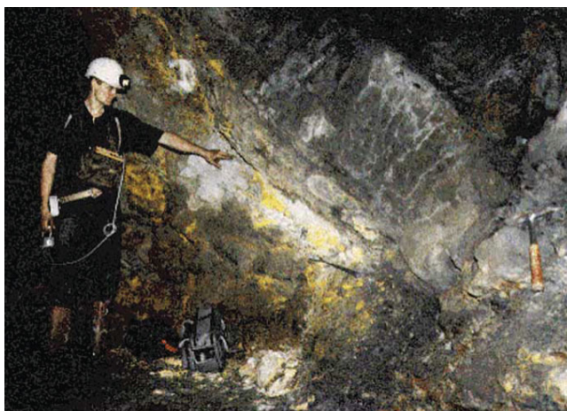
Figure 24.6.1: A “Fossil Nuclear Reactor” in a Uranium Mine Near Oklo in Gabon, West Africa. More than a billion years ago, a number of uranium-rich deposits in West Africa apparently “went critical,” initiating uncontrolled nuclear fission reactions that may have continued intermittently for more than 100,000 years, until the concentration of uranium-235 became too low to support a chain reaction. This photo shows a geologist standing in a mine dug to extract the concentrated uranium ore. Commercial interest waned rapidly after it was recognized that the uranium ore was severely depleted in uranium-235, the isotope of interest.
