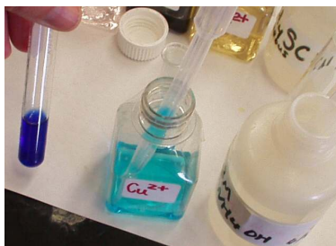
Figure 17.4.1: The Formation of Complex Ions. An aqueous solution of \text{CuSO}_4 consists of hydrated \text{Cu}^{2+} ions in the form of pale blue [\text{Cu}(\text{H}_2\text{O})_6]^{2+} (left). The addition of aqueous ammonia to the solution results in the formation of the intensely blue-violet [\text{Cu}(\text{NH}_3)_4(\text{H}_2\text{O})_2]^{2+} ions, usually written as [\text{Cu}(\text{NH}_3)_4]^{2+} ion (right) because ammonia, a stronger base than \text{H}_2\text{O} , replaces water molecules from the hydrated \text{Cu}^{2+} ion. For a more complete description, see https://www.youtube.com/watch?v=IQNcLH6OZK0 .
