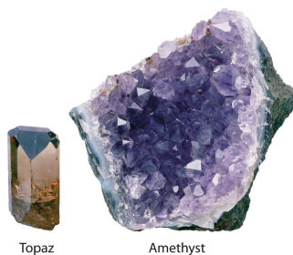
The same cation in different environments. An \text{Fe}^{3+} substitutional impurity produces substances with strikingly different colors.
