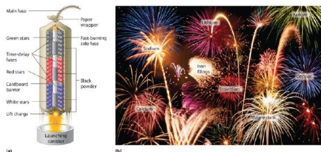
Figure 2.3.9 The Chemistry of Fireworks (a) In the “multibreak” shell used for fireworks, the chambers contain mixtures of fuels and oxidizers plus compounds for special effects (“stars”) connected by time-delay fuses so that the chambers explode in stages. (b) The finale of a fireworks display usually consists of many shells fired simultaneously to give a dazzling multicolor display. The labels indicate the substances that are responsible for the colors of some of the fireworks shown.
