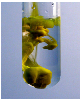
Figure 17.5.2 When a small amount of \text{Na}_2\text{CrO}_4 solution is added to a sample containing \text{Pb}^{2+} ions in water, a bright yellow precipitate of \text{PbCrO}_4 forms. from Wikipedia.
