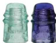
Figure 24.3.1 Radiation Damage When high-energy particles emitted by radioactive decay interact with matter, they can break bonds or ionize molecules, resulting in changes in physical properties such as ductility or color. The glass electrical insulator on the left has not been exposed to radiation, but the insulator on the right has received intense radiation doses over a long period of time. Radiation damage changed the chemical structure of the glass, causing it to become bright blue.
