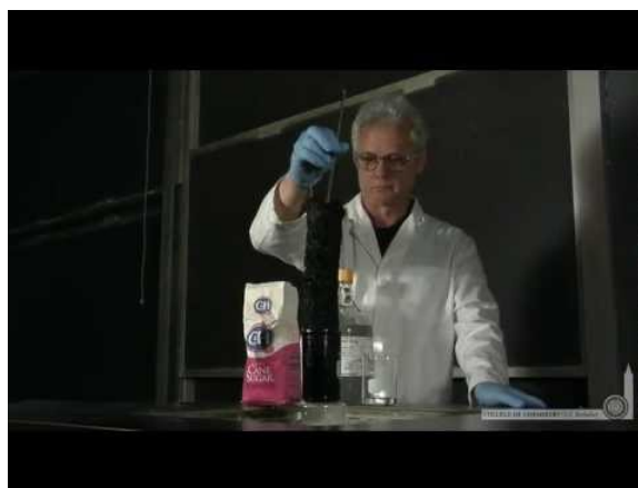
Figure 14.1.1 The Effect of Concentration on Reaction Rates Mixing sucrose with dilute sulfuric acid in a beaker (a, right) produces a simple solution. Mixing the same amount of sucrose with concentrated sulfuric acid (a, left) results in a dramatic reaction (b) that eventually produces a column of black porous graphite (c) and an intense smell of burning sugar.
