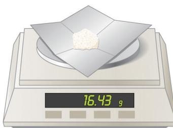
A **balance** is used to measure mass.
