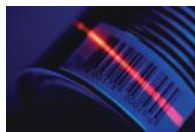
Figure 2.2.4 A Beam of Red Light Emitted by a Helium Neon laser reads a bar code. Originally Helium neon lasers, which emit red light at a wavelength of 632.8 nm, were used to read bar codes. Today, smaller, inexpensive diode lasers are used.
