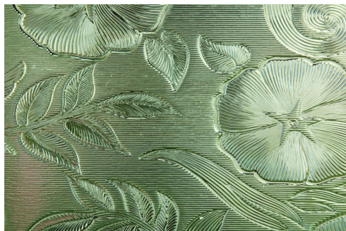
Glass etched with hydrogen fluoride. © Thinkstock
