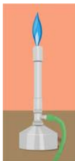
Figure 10.1.3: A Bunsen burner is commonly used to heat substances in a chemistry lab. Methane is reacted with oxygen to form carbon dioxide and water. (Credit: CK-12 Foundation; Source: CK-12 Foundation; License: CK-12 Curriculum Materials license)
