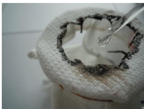
Figure 12.1.1.1: Drops of concentrated sulfuric acid rapidly decompose a piece of cotton towel by dehydration. (CC BY-SA 3.0; Toxic Walker).
