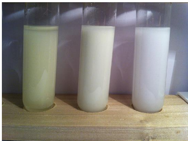
Figure 10.6.1: The three common silver halide precipitates: \text{AgI} , \text{AgBr} and \text{AgCl} (left to right). The silver halides precipitate out of solution, but often form suspensions before settling. (CC BY-SA 3.0; Cychr).
