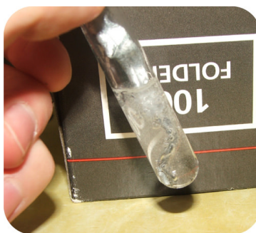
Figure 10.4.4.2: Zinc metal reacts with hydrochloric acid to give off hydrogen gas in a single-displacement reaction. (Credit: User: Chemicalinterest/Wikimedia Commons; Source: http://commons.wikimedia.org/wiki/File:Zn_reaction_with_HCl.JPG (opens in new window); License: Public Domain)
