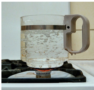
Figure 7.6.1.1: The Boiling Point of Water. Nucleate boiling of water over a kitchen stove burner. (Source: Wikipedia). Water is a good substance to use as an example because many people are already familiar with it. Other substances have melting points and boiling points as well.
