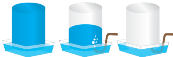
Figure 8.6.2: A gas produced in a chemical reaction can be collected by water displacement.
