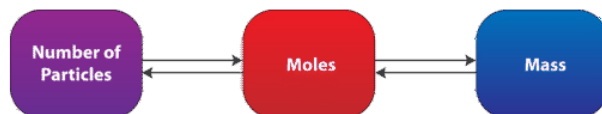
Figure 5.5.1: Conversion from number of particles to mass, or from mass to number of particles requires two steps.
