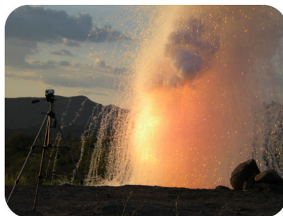
Figure 10.4.4.3: Sodium metal reacts vigorously with water, giving off hydrogen gas. A large piece of sodium will often generate so much heat that the hydrogen will ignite. (Credit: User:Ajhalls/Wikimedia Commons; Source: http://commons.wikimedia.org/wiki/File:Large_Sodium_Explosion.jpg (opens in new window); License: Public Domain)
