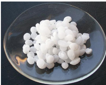
Figure 12.1.2.1: Sample of sodium hydroxide as pellets in a watch glass. (Public Domain; Walkerma.)
