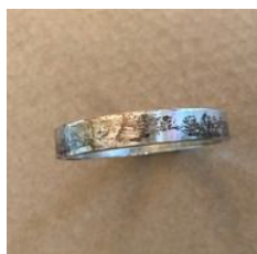
Figure 10.1.2: You can see dark spots of tarnished (silver sulfide) forming on this ring as it reacts with sulfur compounds in the air. (Credit: CK-12 Foundation; Source: CK-12 Foundation; License: CK-12 Curriculum Materials license)
