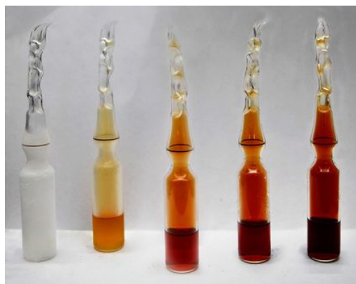
Figure 13.2.1: Dinitrogen tetroxide is a powerful oxidizer that reacts spontaneously upon contact with various forms of hydrazine, which makes the pair a popular propellant combination for rockets. Nitrogen dioxide at -196\text{ }^{\circ}\text{C} , 0\text{ }^{\circ}\text{C} , 23\text{ }^{\circ}\text{C} , 35\text{ }^{\circ}\text{C} , and 50\text{ }^{\circ}\text{C} . ( \text{NO}_2 ) converts to the colorless dinitrogen tetroxide ( \text{N}_2\text{O}_4 ) at low temperatures, and reverts to \text{NO}_2 at higher temperatures. (CC BY-SA 3.0; Eframgoldberg ).
