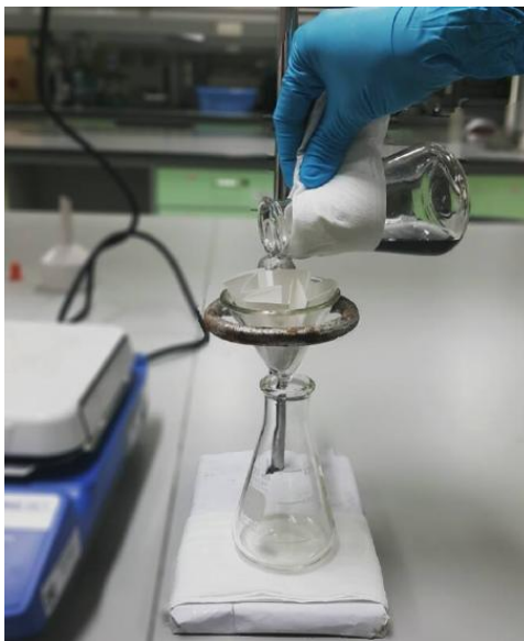
Figure 4.1.2.4: Filtration for the separation of solids from a hot solution. (CC BY-SA 4.0; Suman6395).
