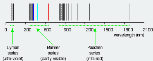
The spectral series of hydrogen based of the Rydberg Equation (on a logarithmic scale).
