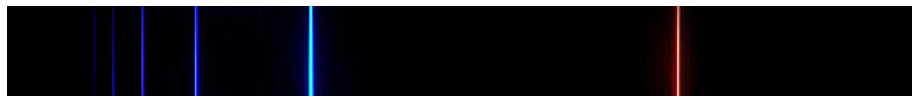
Figure 11.4.4: The visible hydrogen emission spectrum lines in the Balmer series. The red line at the right is the H_{\alpha} line and the two leftmost lines are considered to be ultraviolet as they have wavelengths less than 400 nm. from Wikipedia.
