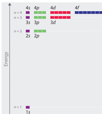
Figure 11.10.7: Orbital Energy Level Diagram for the Hydrogen Atom. Each box corresponds to one orbital. Note that the difference in energy between orbitals decreases rapidly with increasing values of n .
