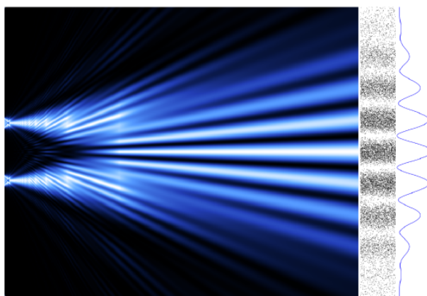
Figure 24.1.2: Numerical simulation of the double-slit experiment with electrons.
