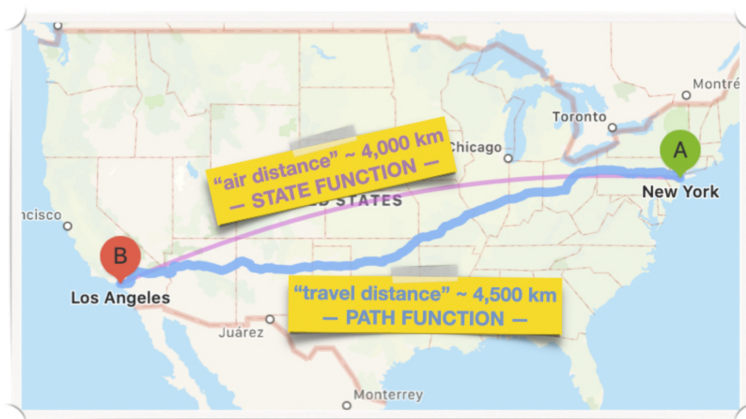
Figure 1.2.1: State Functions vs. Path Functions.
