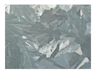
Crystalline surface of a hot-dip galvanized steel surface. This served both as prophylactic protection (protecting the underlying steel from the oxygen in the air) and cathodic protection (once exposed, the zinc will oxidize before the underlying steel).
