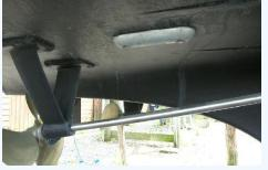
Zinc sacrificial anode (rounded object screwed to underside of hull) used to prevent corrosion on the screw in a boat via cathodic protection. Image by Rémi Kaupp and used with permission.
