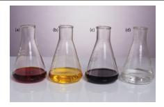
**Figure 9.41** Endpoint for the determination of the total chlorine residual. (a) Acidifying the sample and adding KI forms a brown solution of  $I_3^-$ . (b) Titrating with  $Na_2S_2O_3$  converts  $I_3^-$  to  $I^-$  with the solution fading to a pale yellow color as we approach the end
