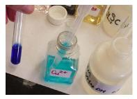
Figure 16.5.1: The Formation of Complex Ions. An aqueous solution of  $CuSO_4$  consists of hydrated  $Cu^{2+}$  ions in the form of pale blue  $[Cu(H_2O)_6]^{2+}$  (left). The addition of aqueous ammonia to the solution results in the formation of the intensely blue-violet  $[Cu(NH_3)_4(H_2O)_2]^{2+}$  ions, usually written as  $[Cu(NH_3)_4]^{2+}$  ion (right) because ammonia, a stronger base than  $H_2O$ , replaces water
