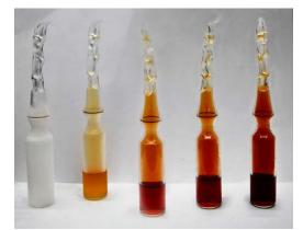
Figure 14.1.1: Dinitrogen tetroxide is a powerful oxidizer that reacts spontaneously upon contact with various forms of hydrazine, which makes the pair a popular propellant combination for rockets. Nitrogen dioxide at -196 °C, 0 °C, 23 °C, 35 °C, and 50 °C. (NO<sub>2</sub>) converts to the colorless dinitrogen tetroxide (N<sub>2</sub>O<sub>4</sub>) at low temperatures, and reverts to NO<sub>2</sub> at higher temperatures. (CC BY-SA 3.0; Eframgoldberg).
