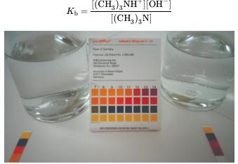
Figure 15.4.2: pH paper indicates that a 0.1-M solution of NH<sub>3</sub> (left) is weakly basic. The solution has a pOH of 3 ( $[OH^-] = 0.001$  M) because the weak base NH<sub>3</sub> only partially reacts with water. A 0.1-M solution of NaOH (right) has a pOH of 1 because NaOH is a strong base (credit: modification of work by Sahar Atwa).
