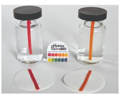
Figure 15.4.1: pH paper indicates that a 0.1-M solution of HCl (beaker on left) has a pH of 1. The acid is fully ionized and  $[H_3O^+] = 0.1 \text{ M}$ . A 0.1-M solution of CH<sub>3</sub>CO<sub>2</sub>H (beaker on right) has a pH of 3 ( $[H_3O^+] = 0.001 \text{ M}$ ) because the weak acid CH<sub>3</sub>CO<sub>2</sub>H is only partially ionized. In this solution,  $[H_3O^+] < [CH_3CO_2H]$ . (credit: modification of work by Sahar Atwa)
