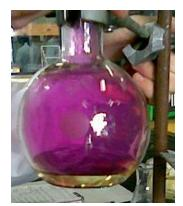
Figure 10.5.2: The Sublimation of solid iodine. When solid iodine is heated at ordinary atmospheric pressure, it sublimes. When the  $I_2$  vapor comes in contact with a cold surface, it deposits  $I_2$  crystals. Figure used with permission from Wikipedia.
