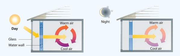
**Passive solar system.** During the day (a), sunlight is absorbed by water circulating in the water wall. At night (b), heat stored in the water wall continues to warm the air inside the house.
