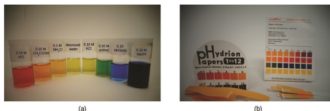
Figure 15.2.5 (a) A universal indicator assumes a different color in solutions of different pH values. Thus, it can be added to a solution to determine the pH of the solution. The eight vials each contain a universal indicator and 0.1-M solutions of progressively weaker acids: HCl (pH = 1), \text{CH}_3\text{CO}_2\text{H} (pH = 3), and \text{NH}_4\text{Cl} (pH = 5), deionized water, a neutral substance (pH = 7); and 0.1-M solutions of the progressively stronger bases: KCl (pH = 7), aniline, \text{C}_6\text{H}_5\text{NH}_2 (pH = 9), \text{NH}_3 (pH = 11), and NaOH (pH = 13). (b) pH paper contains a mixture of indicators that give different colors in solutions of differing pH values. (credit: modification of work by Sahar Atwa).
