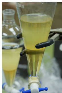
Figure 14.8.2: A separatory funnel with two solvents.
