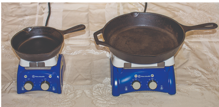
Figure 12.3.1: Due to its larger mass, a large frying pan has a larger heat capacity than a small frying pan. Because they are made of the same material, both frying pans have the same specific heat. (CC BY; Mark Blaser via OpenStax).
