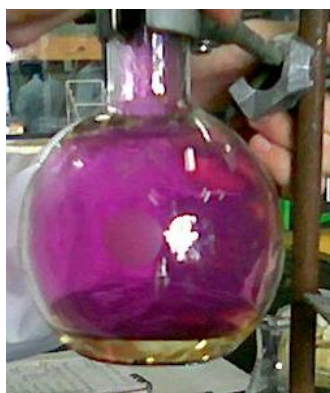
Figure 10.5.2: The Sublimation of solid iodine. When solid iodine is heated at ordinary atmospheric pressure, it sublimates. When the I 2 vapor comes in contact with a cold surface, it deposits I 2 crystals. Figure used with permission from Wikipedia.
