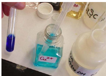
Figure 16.5.1: The Formation of Complex Ions. An aqueous solution of \text{CuSO}_4 consists of hydrated \text{Cu}^{2+} ions in the form of pale blue [\text{Cu}(\text{H}_2\text{O})_6]^{2+} (left). The addition of aqueous ammonia to the solution results in the formation of the intensely blue-violet [\text{Cu}(\text{NH}_3)_4(\text{H}_2\text{O})_2]^{2+} ions, usually written as [\text{Cu}(\text{NH}_3)_4]^{2+} ion (right) because ammonia, a stronger base than \text{H}_2\text{O} , replaces water molecules from the hydrated \text{Cu}^{2+} ion. For a more complete description, see www.youtube.com/watch?v=IQNcLH6OZK0 .
