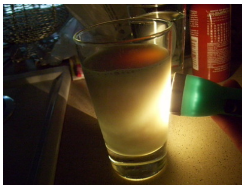
Figure 11.7.1: Tyndall Effect, the Scattering of Light by Colloids (CC BY; LibreTexts)
