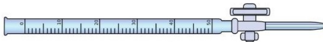
Figure 5.13.1: Equipment for Titrations. A burette is a type of liquid dispensing system that can accurately indicate the volume of liquid dispensed.
