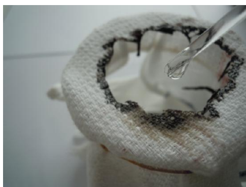
Figure 5.8.1: Drops of concentrated sulfuric acid rapidly decompose a piece of cotton towel by dehydration. (CC BY-SA 3.0; Toxic Walker).
