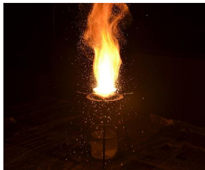
Figure 10.3.3: The thermite reaction produces so much heat that the iron it produces comes out molten, a property that makes this reaction useful in welding. Image by Kingfisher [CC BY-SA 3.0 ( Creative Commons [creativecommons.org])], from Wikimedia Commons.
