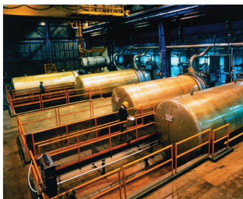
Figure A Portion of a Plant for Separating Uranium Isotopes by Effusion of \text{UF}_6 . The large cylindrical objects (note the human for scale) are so-called diffuser (actually effuser) units, in which gaseous \text{UF}_6 is pumped through a porous barrier to partially separate the isotopes. The \text{UF}_6 must be passed through multiple units to become substantially enriched in ^{235}\text{U} .
