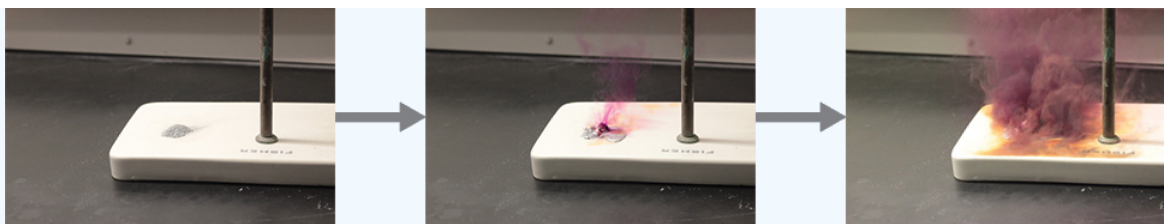
Figure 8.4.1: Aluminum and iodine react to produce aluminum iodide. The heat of the reaction vaporizes some of the solid iodine as a purple vapor. (credit: modification of work by Mark Ott)
