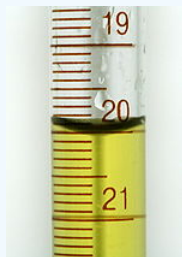
Figure 2.2.2: A meniscus as seen in a burette of colored water.
