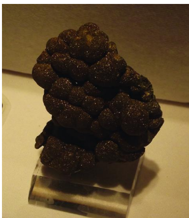
Figure 23.2.8: Blister copper is obtained during the conversion of copper-containing ore into pure copper. (credit: "Tortie tude"/Wikimedia Commons)
