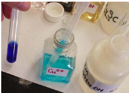
Figure 14.7.3: The Formation of Complex Ions. An aqueous solution of \text{CuSO}_4 consists of hydrated \text{Cu}^{2+} ions in the form of pale blue [\text{Cu}(\text{H}_2\text{O})_6]^{2+} (left). The addition of aqueous ammonia to the solution results in the formation of the intensely blue-violet [\text{Cu}(\text{NH}_3)_4(\text{H}_2\text{O})_2]^{2+} ions, usually written as [\text{Cu}(\text{NH}_3)_4]^{2+} ion (right) because ammonia, a stronger base than \text{H}_2\text{O} , replaces water molecules from the hydrated \text{Cu}^{2+} ion. For a more complete description, see www.youtube.com/watch?v=IQNcLH6OZK0 .
