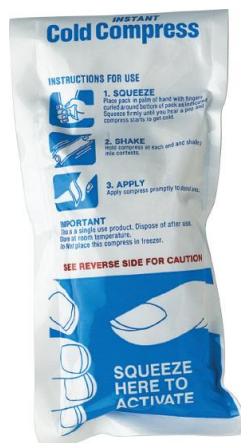
Figure 14.2.3: Commercial Cold Packs for Treating Injuries. These packs contain solid \text{NH}_4\text{NO}_3 and water in separate compartments. When the seal between the compartments is broken, the \text{NH}_4\text{NO}_3 dissolves in the water. Because \Delta H_{\text{soln}} for \text{NH}_4\text{NO}_3 is much greater than zero, heat is absorbed by the cold pack during the dissolution process, producing local temperatures less than 0^\circ\text{C} .
