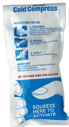
Figure 14.3.3: Commercial Cold Packs for Treating Injuries. These packs contain solid NH_4NO_3 and water in separate compartments. When the seal between the compartments is broken, the NH_4NO_3 dissolves in the water. Because \Delta H_{soln} for NH_4NO_3 is much greater than zero, heat is absorbed by the cold pack during the dissolution process, producing local temperatures less than 0°C.
