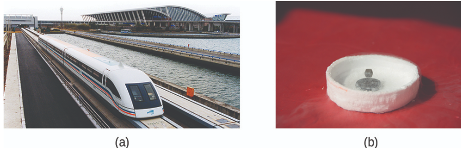
Figure 23.2.11: (a) This magnetic levitation train (or maglev) uses superconductor technology to move along its tracks. (b) A magnet can be levitated using a dish like this as a superconductor. (credit a: modification of work by Alex Needham; credit b: modification of work by Kevin Jarrett)
