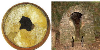
Figure 14.4.3: Calcium carbonate deposits (left) Calcium carbonate ( \text{CaCO}_3 ) deposits in hot water pipes can significantly reduce pipe capacity. These deposits, called boiler scale, form when dissolved \text{CO}_2 is driven into the gas phase at high temperatures. (right) Highly calcified remains of Eiffel aqueduct near Euskirchen-Kreuzweingarten, Germany. (Wikipedia)
