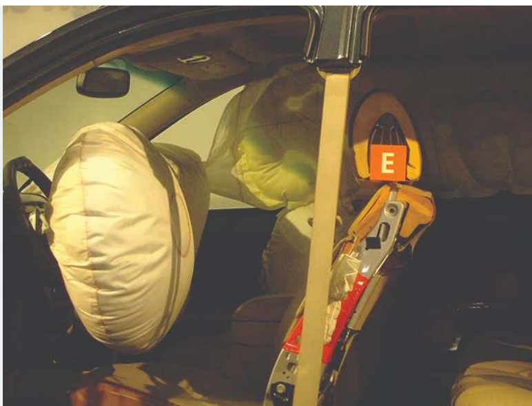
Figure 8.5.3: Airbags deploy upon impact to minimize serious injuries to passengers. (credit: Jon Seidman)
