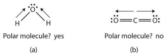
Figure 4.5.7 Physical Properties and Polarity. The physical properties of water and carbon dioxide are affected by their polarities.
