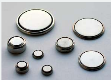
Figure 5.6.1: A small button battery like this is used to power a watch, pacemaker, or calculator. (CC BY-SA; Gerhard H Wrodnigg via Wikipedia )
