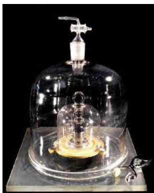
Figure 1.7.1: The Kilogram. The standard for the kilogram is a platinum-iridium cylinder kept in a special vault in France. Source: Photo reproduced by permission of the Bureau International des Poids et Mesures, who retain full internationally protected copyright.
