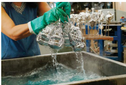
Figure 13.11.1: Aldehyde Reactions. A reaction related to the Tollens' reaction is often used to silver mirrors. These ornaments were silvered by such a reaction. Glucose, a simple sugar with an aldehyde functional group, is used as the reducing agent. Source: Photo courtesy of Krebs Glas Lauscha, commons.wikimedia.org/wiki/File:Silvering.jpg.
