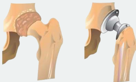
Figure 12.6.1: Hip Joint Replacement. Synthetic polymers are an important part of a hip joint replacement. The hip is much like a ball-and-socket joint, and total hip replacements mimic this with a metal ball that fits in a plastic cup.
