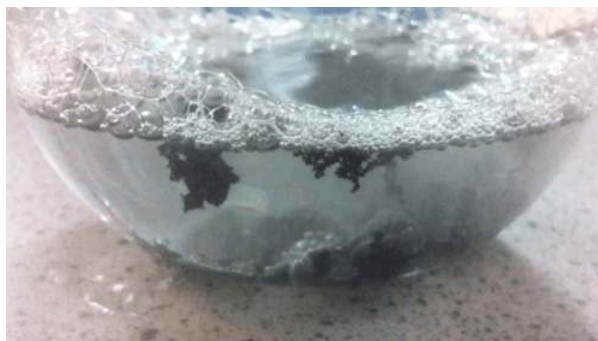
Figure 5.6.1: Zinc Metal plus Hydrochloric Acid. It is fairly obvious that zinc metal reacts with aqueous hydrochloric acid! The bubbles are hydrogen gas (right side of Equation 5.6.1).
