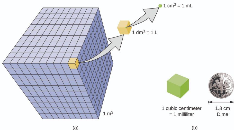
Figure 1.7.3: Units of Volume. (a) The relative volumes are shown for cubes of  $1 \text{ m}^3$ ,  $1 \text{ dm}^3$  (1 L), and  $1 \text{ cm}^3$  (1 mL) (not to scale). A liter (L) is defined as a cube 1 dm (1/10th of a meter) on a side. A milliliter (mL), 1/1,000th of a liter, is equal to 1 cubic centimeter. (b) The diameter of a dime is compared relative to the edge length of a  $1\text{-cm}^3$  (1-mL) cube. (CC BY 4.0; OpenStax)
