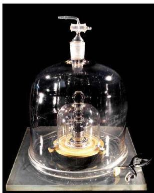
Figure 1.7.1: The Kilogram. The standard for the kilogram is a platinum-iridium cylinder kept in a special vault in France. Source: Photo reproduced by permission of the Bureau International des Poids et Mesures, who retain full internationally protected copyright.
