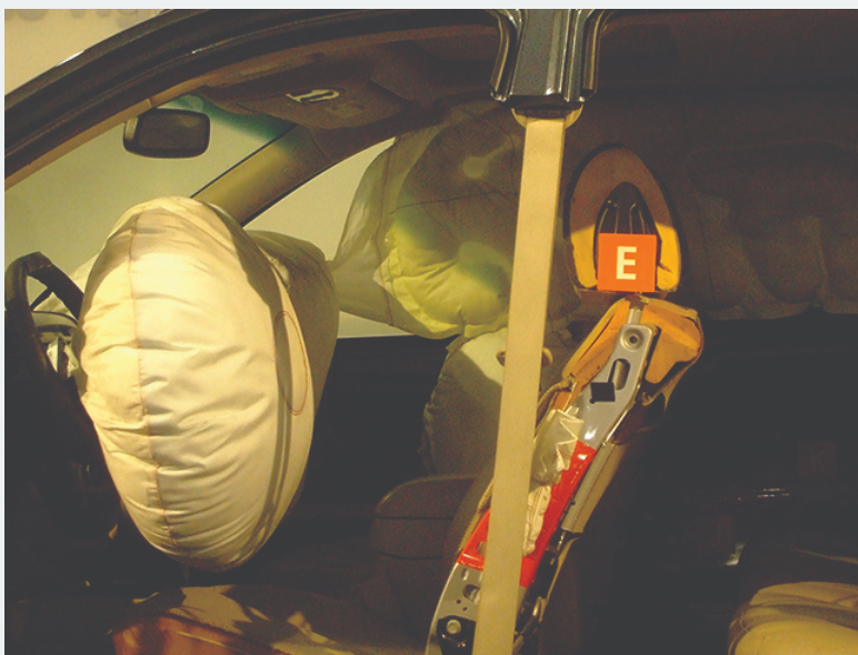
Figure 9.5.3: Airbags deploy upon impact to minimize serious injuries to passengers. (credit: Jon Seidman)
