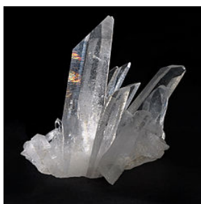
Figure 9.3.1: Crystalline Arrangement of Quartz crystal cluster. Some large crystals look the way they do because of the regular arrangement of atoms (ions) in their crystal structure. from Wikipedia.
