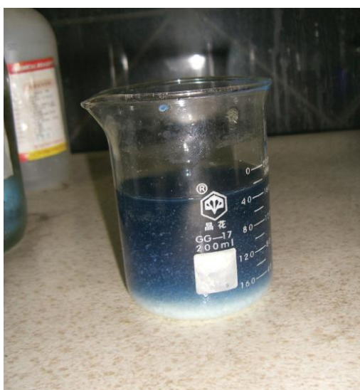
Figure 7.5.2: Double-Replacement Reactions. Some double-replacement reactions are obvious because you can see a solid precipitate coming out of solution. Source: Photo courtesy of Chojj, Wikimedia (opens in new window) [commons.wikimedia.org].
