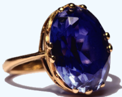
Figure 5.1.8.2: Although pure aluminum oxide is colorless, trace amounts of iron and titanium give blue sapphire its characteristic color. (credit: modification of work by Stanislav Doronenko)
