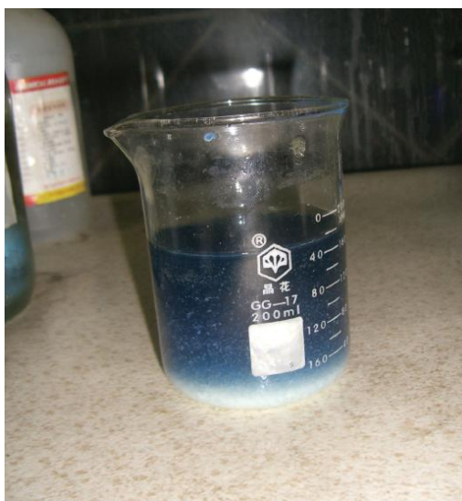
Figure 7.5.2: Double-Replacement Reactions. Some double-replacement reactions are obvious because you can see a solid precipitate coming out of solution. Source: Photo courtesy of Choi, Wikimedia (opens in new window) [commons.wikimedia.org].
