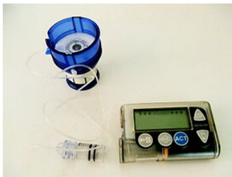
Figure 15.1.1: Insulin pump, showing an infusion set loaded into spring-loaded insertion device. A reservoir is attached to the infusion set (shown here removed from the pump). (Public Domain; User:David-i98 ).
