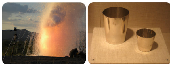
Figure 16.5.1: On the left, sodium reacts with water. On the right, silver in the form of cups do not react with water.
