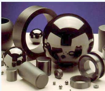
Figure 6.4.2: \text{Si}_3\text{N}_4 bearing parts. (Public Domain; David W. Richerson and Douglas W. Freitag; Oak Ridge National Laboratory).
