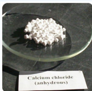
Figure 6.4.3: Calcium chloride is used as a drying agent and as a road deicer.
