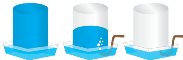
Figure 11.9.2: A gas produced in a chemical reaction can be collected by water displacement.
