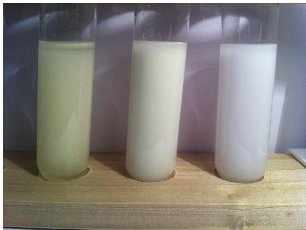
Figure 7.7.1: The three common silver halide precipitates: \text{AgI} , \text{AgBr} and \text{AgCl} (left to right). The silver halides precipitate out of solution, but often form suspensions before settling. (CC BY-SA 3.0; Cychr).
