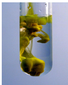
Figure 7.10.3: Lead (II) iodide precipitates when potassium iodide is mixed with lead (II) nitrate (Equation 7.10.1). (CC BY-SA 3.0; PRHaney).
