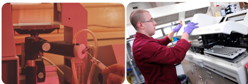
Figure 1.7.2: (left) Measurement of trace metals using atomic spectroscopy. (right) Measurement of hormone concentrations.
