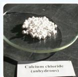
Figure 8.2.3: Calcium chloride is used as a drying agent and as a road deicer.
