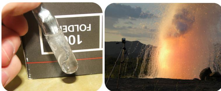
Figure 9.4.2: (First image) Zinc metal reacts with hydrochloric acid to give off hydrogen gas in a single-displacement reaction. (Second image) Sodium metal reacts vigorously with water, giving off hydrogen gas. A large piece of sodium will often generate so much heat that the hydrogen will ignite.
