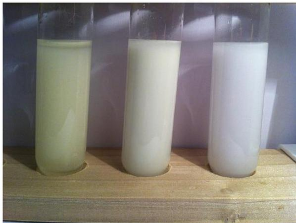
Figure 9.8.1: The three common silver halide precipitates:  $\text{AgI}$ ,  $\text{AgBr}$  and  $\text{AgCl}$  (left to right). The silver halides precipitate out of solution, but often form suspensions before settling. (CC BY-SA 3.0; Cychr).
