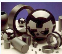
Figure 8.2.2:  $\text{Si}_3\text{N}_4$  bearing parts. (Public Domain; David W. Richerson and Douglas W. Freitag; Oak Ridge National Laboratory).
