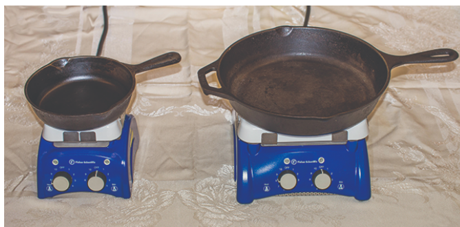
Figure 2.8.7: Due to its larger mass, a large frying pan has a larger heat capacity than a small frying pan. Because they are made of the same material, both frying pans have the same specific heat. (credit: Mark Blaser).
